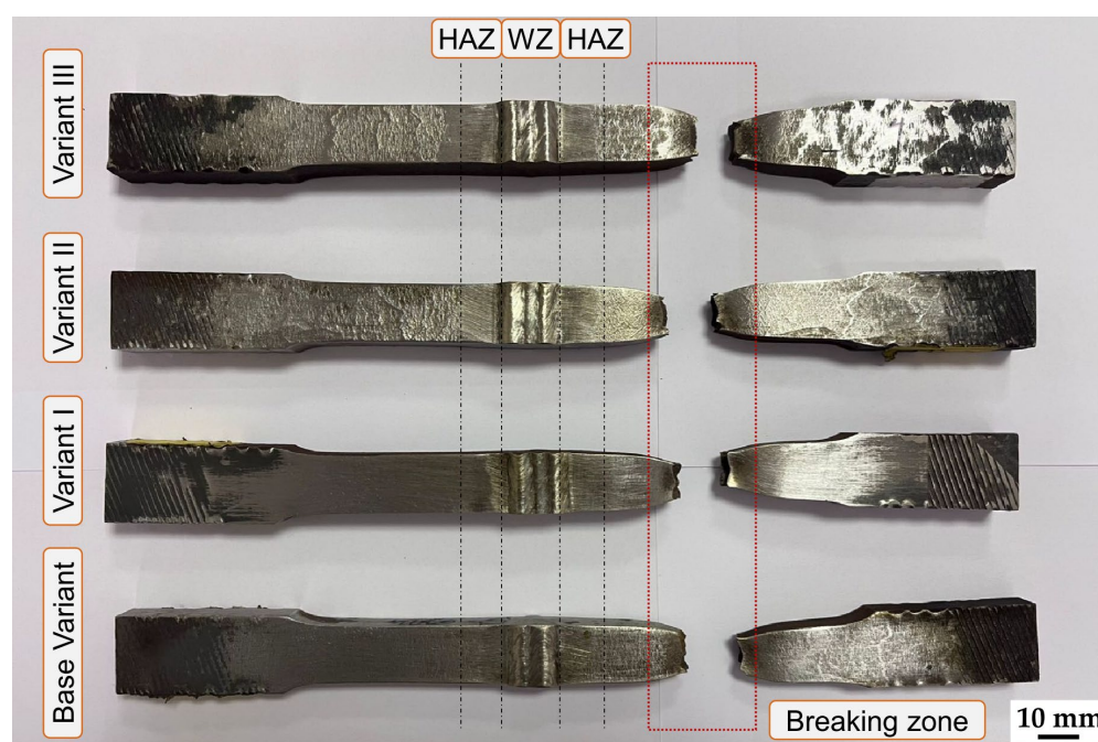
Figure 16. Welded samples after the tensile test.
