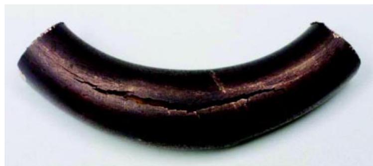
**Figure 21.** Photo of the copper tube failure studied by McDougal and Stevenson reprinted with permission from ref. [57] Springer Nature BV, 2004.
