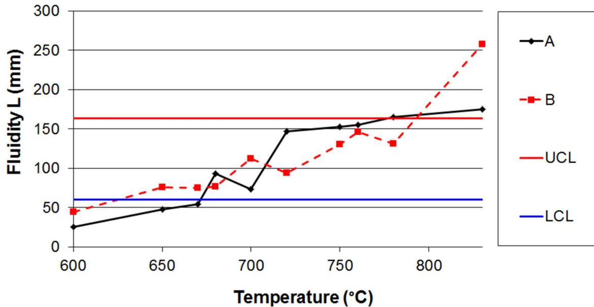
**Figure 4.** X—bar control chart; operators A and B; UCL (upper standard limit) and LSL (lower standard limit).
