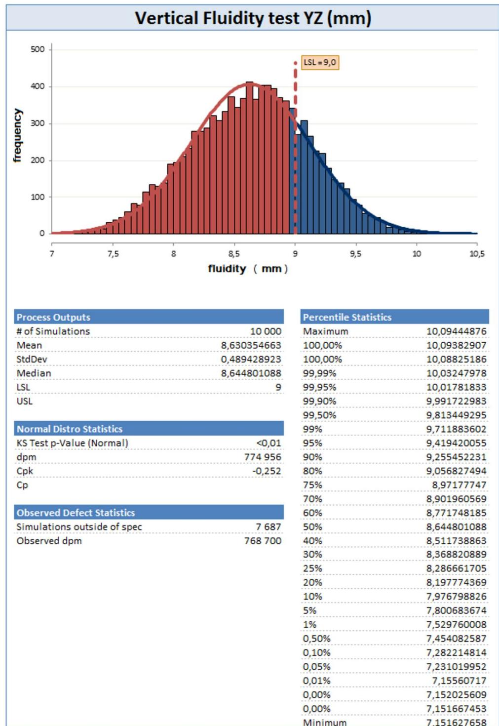
**Figure 8.** Monte Carlo method for the “vertical” mold. Blue color—data within satisfactory tolerance limits. Red color—data within unsatisfactory tolerance limits.
