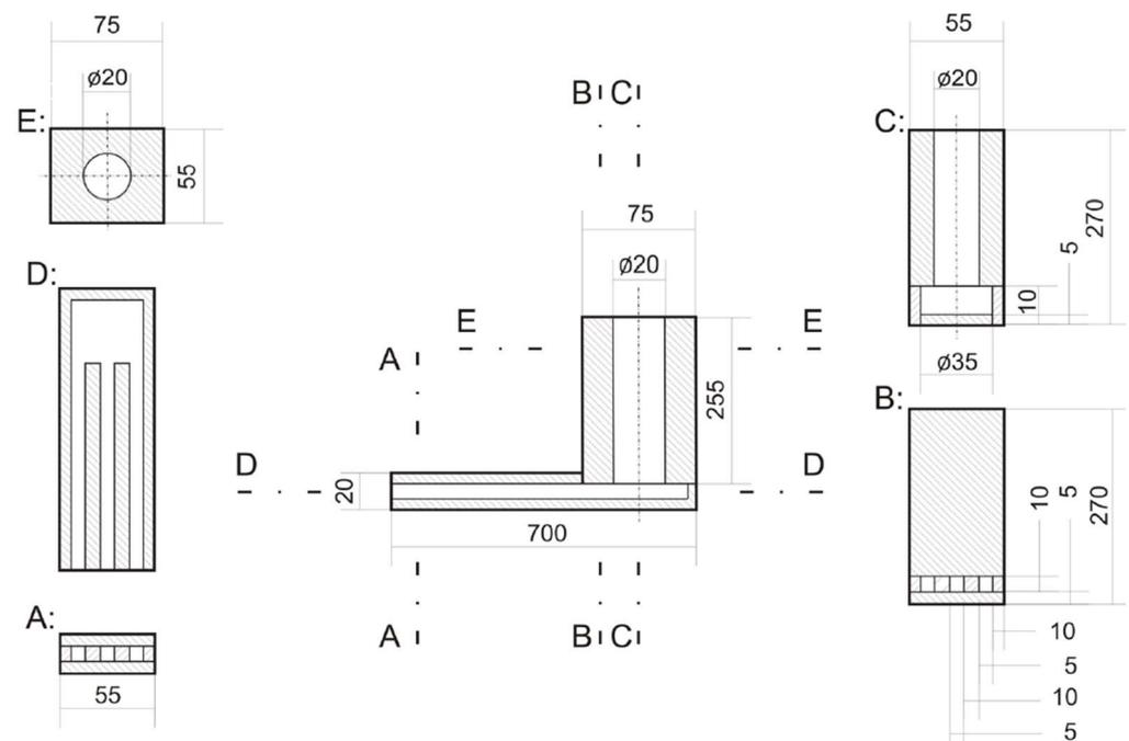
**Figure 1.** Drawing of the “horizontal” mold (the dimensions are in mm). Axes of the cut from different views (A–E).
