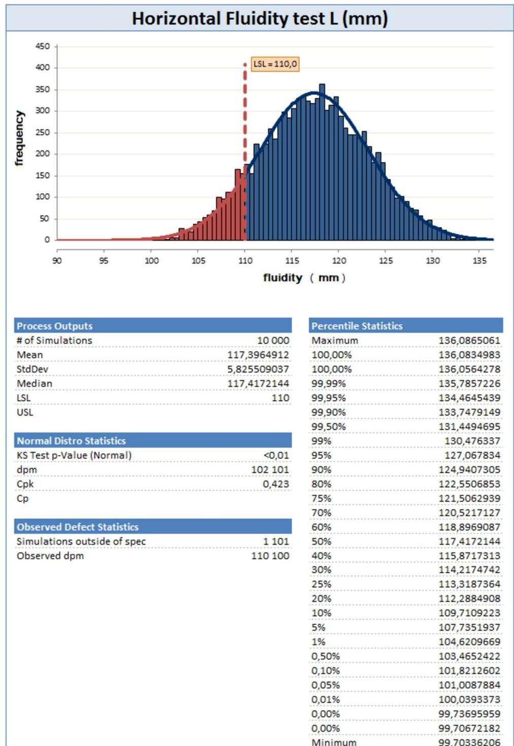
Figure 7. Monte Carlo method for the “horizontal” mold.
