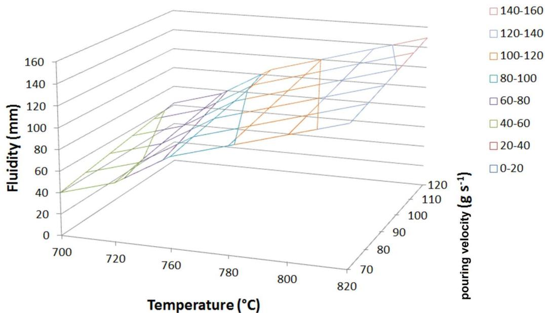
**Figure 6.** “Horizontal” mold pre-heated to 120 °C; dependence of fluidity on the temperature of the mold and pouring velocity.
