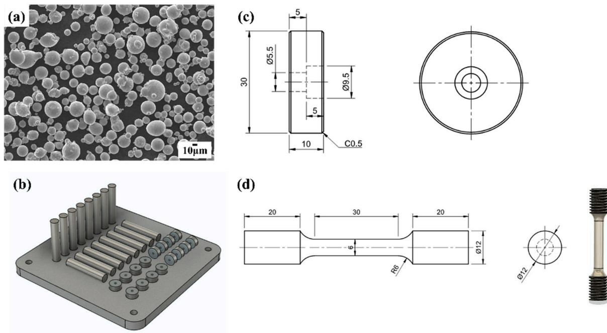
**Figure 1.** (a) SEM image of powdered Ni-based superalloy Inconel 718, (b) schematics of two stacking orientations (horizontal, vertical) for analysis specimens and tensile specimens, (c) schematic of analysis specimen specifications, and (d) schematic of tensile specimen specifications and helical machining shape.
