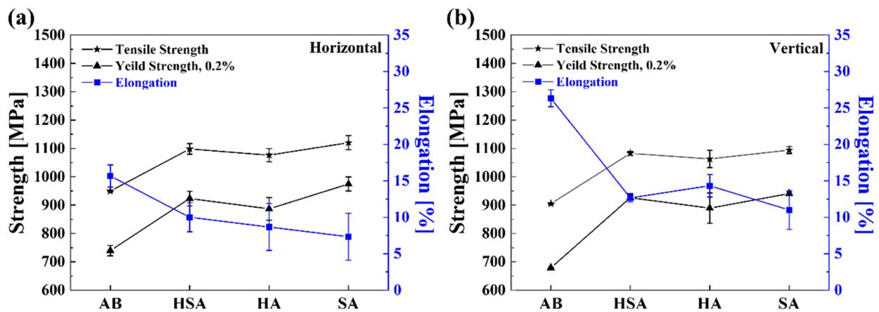
**Figure 8.** High-temperature (650 °C) tensile properties of Inconel 718 alloy manufactured by SLM based in the horizontal (a) and vertical (b) building directions under different heat treatment conditions.
