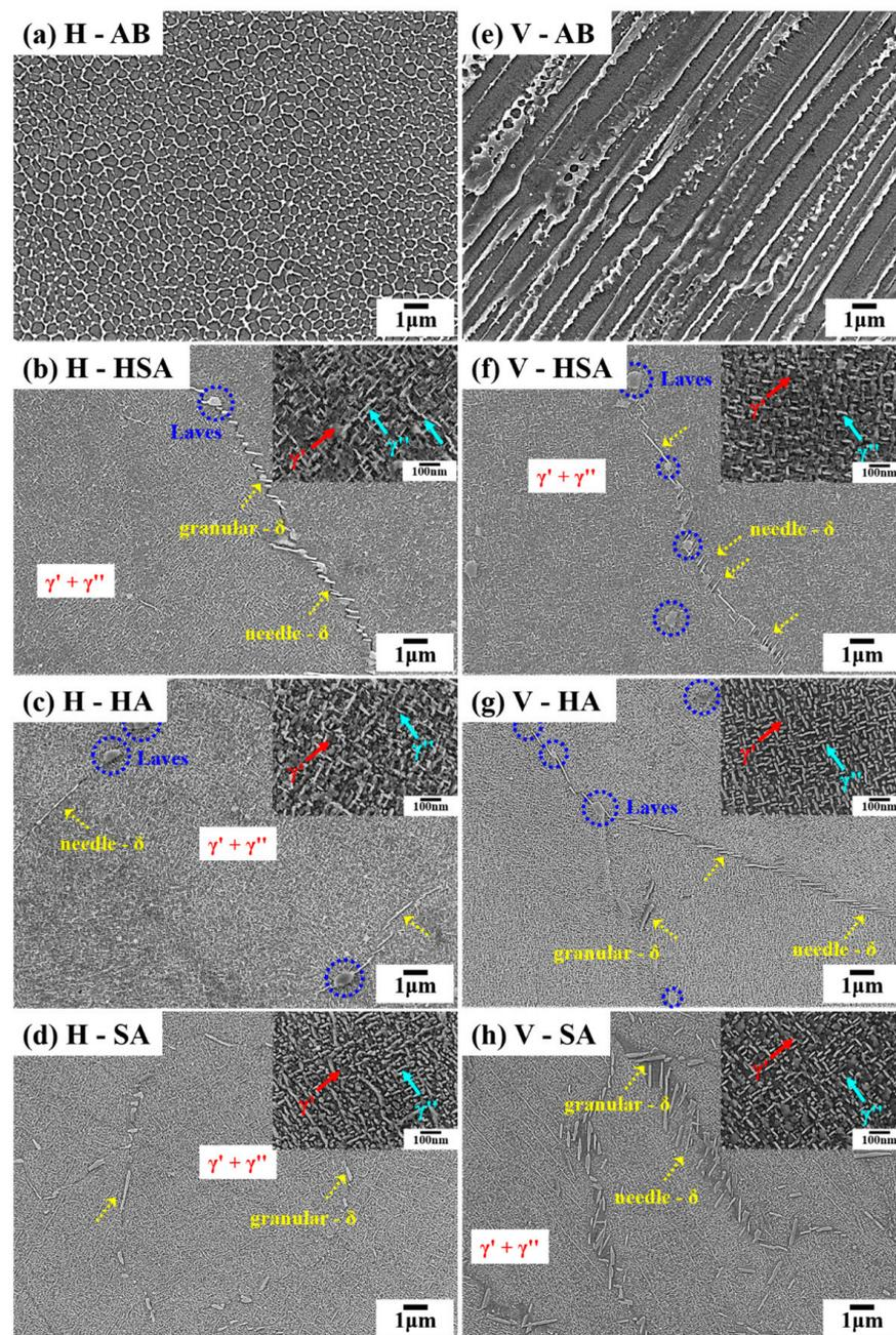
**Figure 4.** The FE-SEM image depicts aligned  $\delta$  precipitates and Laves phase in the building direction. Additionally, higher magnification images reveal the presence of  $\gamma'$  and  $\gamma''$  phases: (a) H-AB, (b) H-HSA, (c) H-HA, (d) H-SA, (e) V-AB, (f) V-HSA, (g) V-HA, and (h) V-SA.
