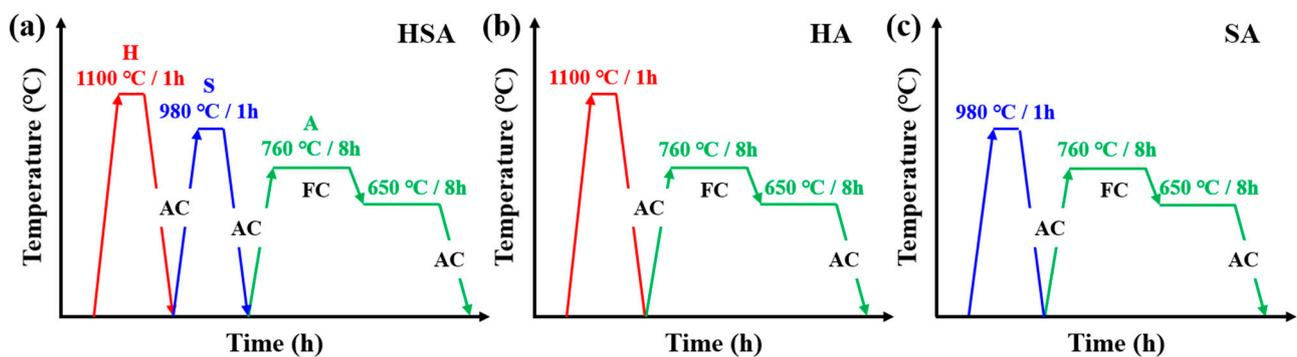
**Figure 2.** Designations of the specimens and the details of the corresponding post-treatment conditions. (a) HSA, (b) HA, and (c) SA.
