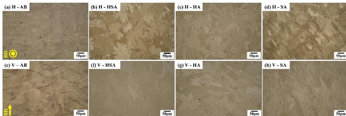
**Figure 3.** Optical microstructure of Inconel 718 with different building directions (BD) and heat treatment conditions of (a) H-AB, (b) H-HSA, (c) H-HA, (d) H-SA, (e) V-AB, (f) V-HSA, (g) V-HA, and (h) V-SA.
