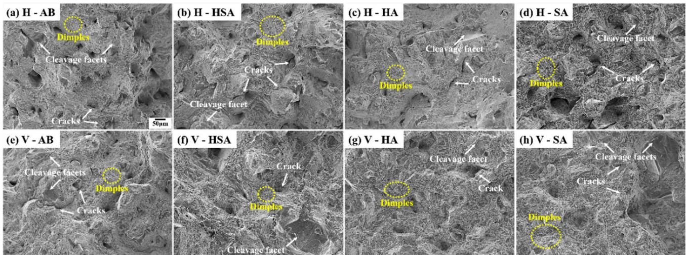
**Figure 9.** SEM microstructure of SLM-produced Inconel 718 alloy after room-temperature tensile fracture, as influenced by heat treatment and building direction: (a) H-AB, (b) H-HSA, (c) H-HA, (d) H-SA, (e) V-AB, (f) V-HSA, (g) V-HA, and (h) V-SA.
