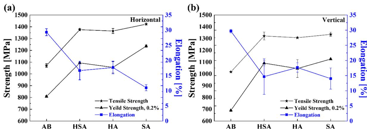
**Figure 7.** The room temperature tensile properties of Inconel 718 alloy manufactured by SLM based on the building direction of (a) horizontal and (b) vertical with various heat treatment conditions.
