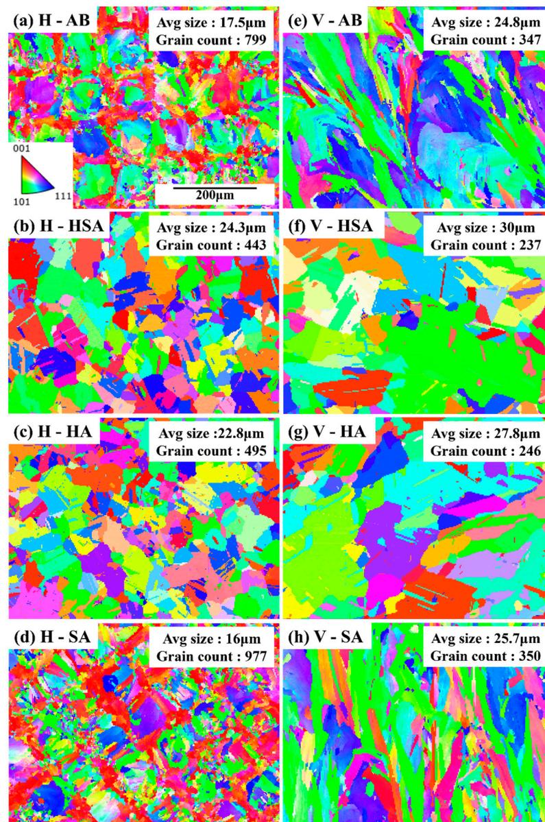
**Figure 5.** EBSD images and the average grain size (in terms of equivalent circle diameter,  $\mu\text{m}$ ) of each specimen as described in the paper: (a) H-AB, (b) H-HSA, (c) H-HA, (d) H-SA, (e) V-AB, (f) V-HSA, (g) V-HA, and (h) V-SA.
