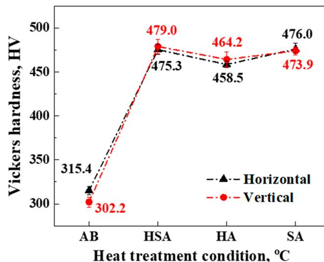
**Figure 6.** Vickers hardness of SLMed Inconel 718 with different building direction and heat conditions.
