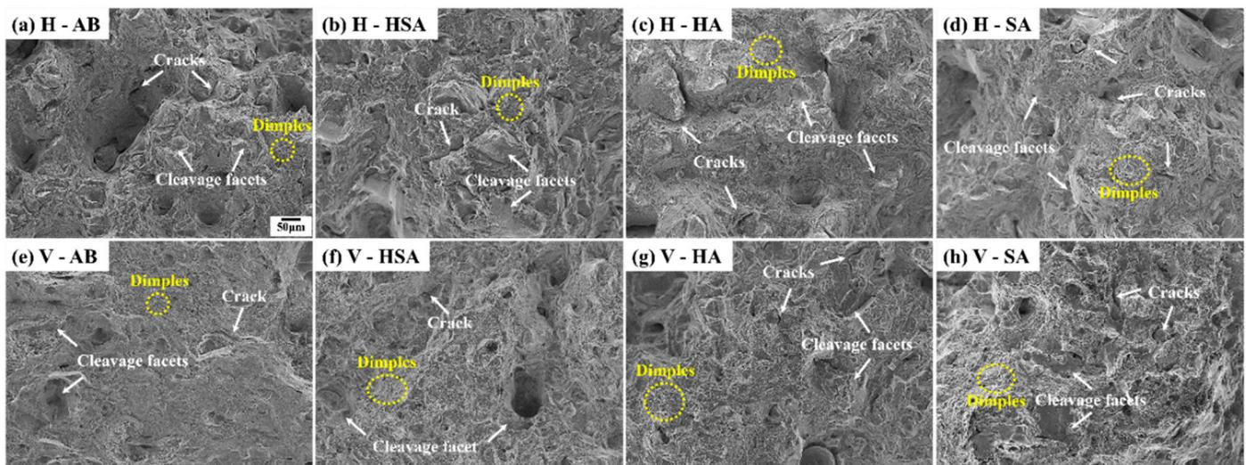
**Figure 10.** SEM microstructure of SLM-produced Inconel 718 alloy after high-temperature tensile fracture (650 °C), as influenced by heat treatment and building direction: (a) H-AB, (b) H-HSA, (c) H-HA, (d) H-SA, (e) V-AB, (f) V-HSA, (g) V-HA, and (h) V-SA.
