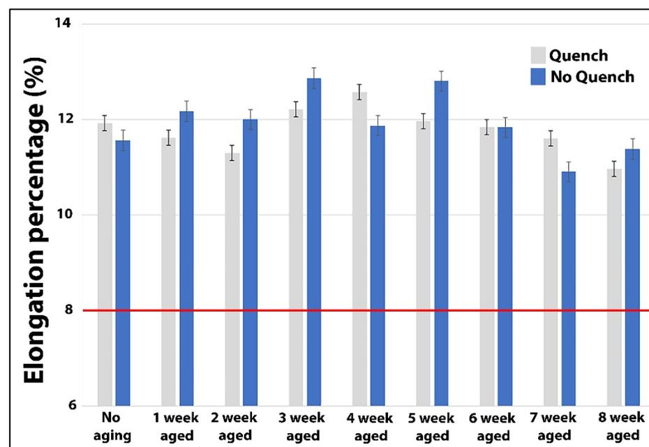
**Figure 4.** Mechanical properties of elongation with and without quenching.
