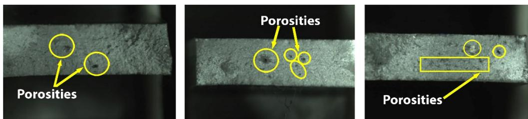
**Figure 7.** Examples of porosity in samples tested for mechanical properties.
