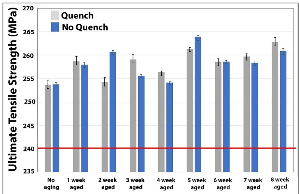
Figure 6. Mechanical properties of tensile strength with and without quenching.
