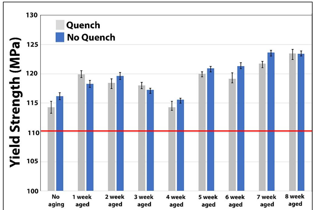
Figure 5. Mechanical properties of yield strength with and without quenching.
