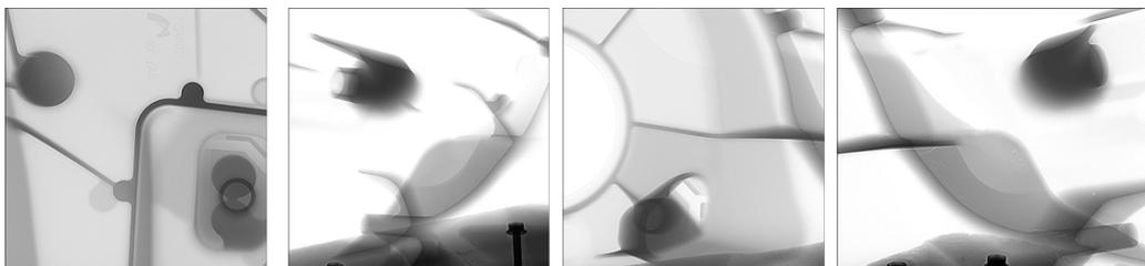
**Figure 8.** Shock towers were analyzed by X-ray technique, showing no porosity or internal defects.
