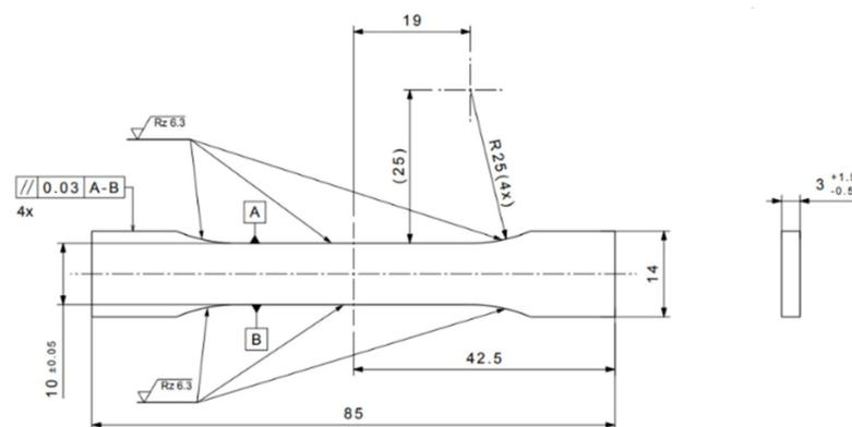
**Figure 2.** Specification of the specimens that were taken from the shock tower (units in mm).
