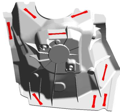
**Figure 3.** Schematic of the Shock tower component showing the position where the tensile coupons were obtained and areas for evaluations.
