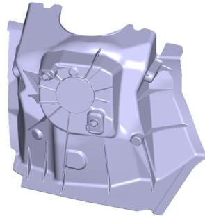
**Figure 1.** Model of the *shock tower* component.
