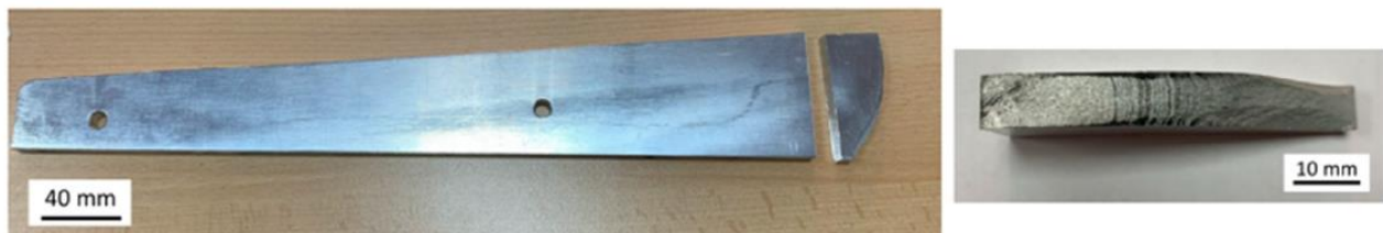
Figure 3. Detail of the extraction of the fracture surface of the cutting system blade.
