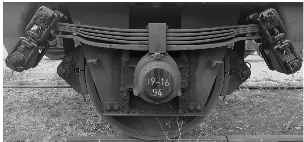
**Figure 1.** Illustration of a parabolic leaf spring in a freight wagon suspension.
