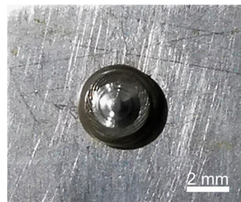
Figure 4. Appearance of 1.5 mm diameter steel ball welded onto 0.6 mm thick sheet.
