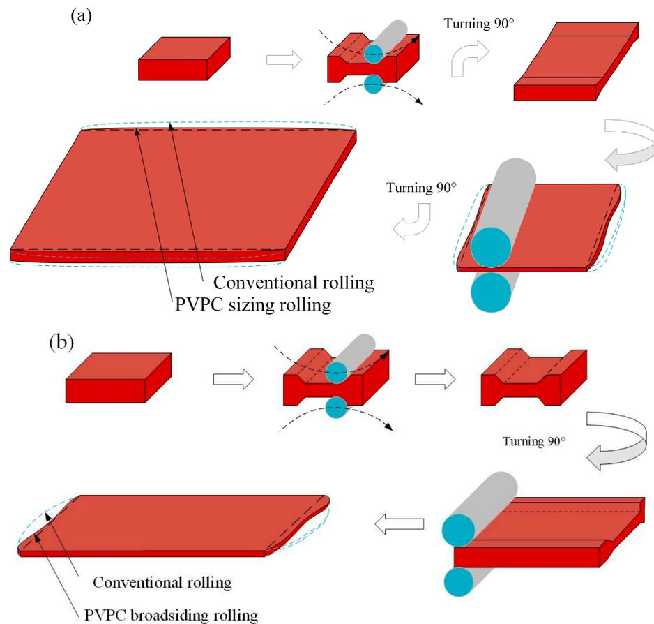
**Figure 1.** Rolling process of PVPC: (a) PVPC sizing rolling, and (b) PVPC broadsiding rolling.
