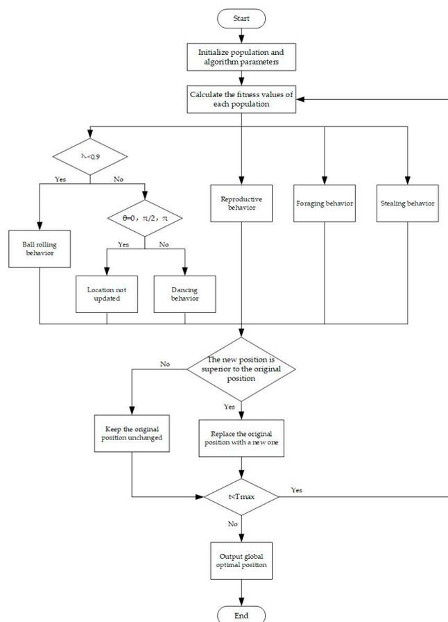
Figure 11. Flow chart of DBO algorithm.
