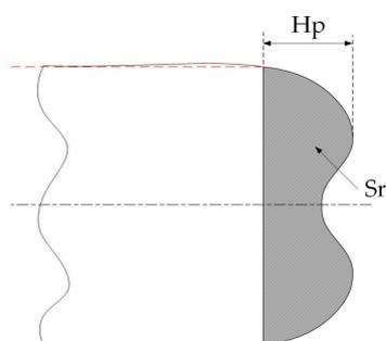
**Figure 9.** Parameter extraction of crop pattern deformation. The black line represents the actual contour of the edges of the rolled steel plate, while the red line represents the contour of the edges of the cut steel plate.
