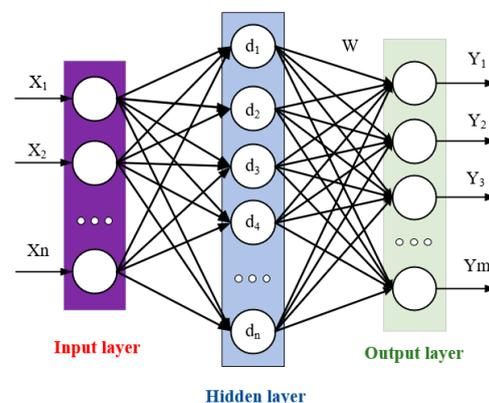
**Figure 10.** Schema of RBF network neural structure.
