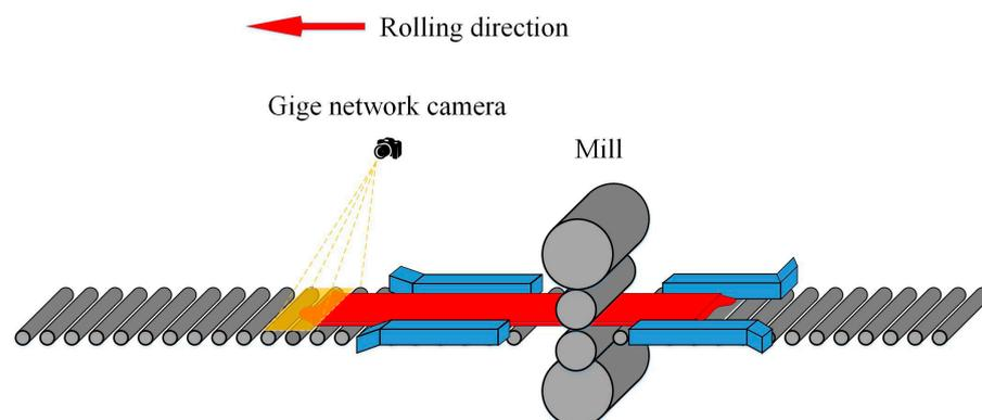
**Figure 2.** Schema of camera installation position.
