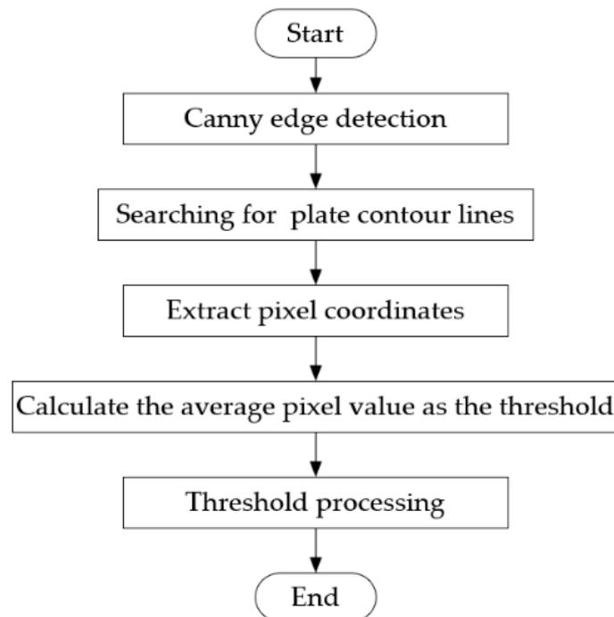
**Figure 4.** Flow chart of automatic threshold adjustment algorithm.
