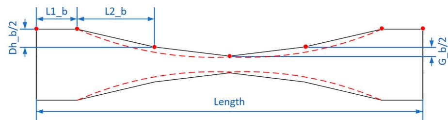
**Figure 8.** Cross section of plate. The red line in the picture represents the contour line of the steel plate after PVPC technology is applied, the black line represents the simplified contour line, and the red points are the feature points set in the seven point control method to define variables.
