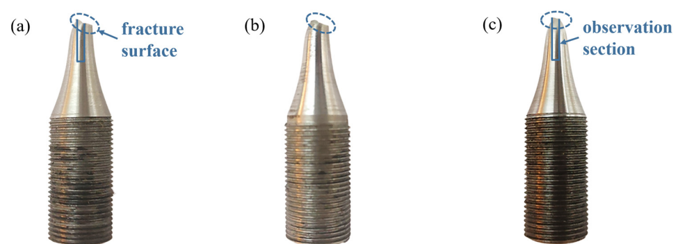
Figure 8. Fatigue specimens at room temperature under different maximum stress levels at (a) 480 MPa, (b) 500 MPa, and (c) 520 MPa.
