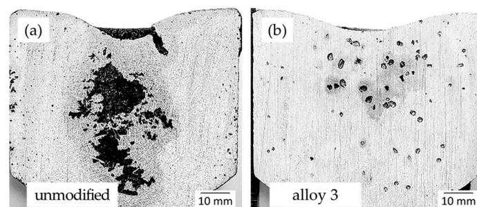
**Figure 6.** The manifestation of volumetric shrinkage in the Al-12wt%Si alloy: (a) unmodified; (b) modified with Rb.
