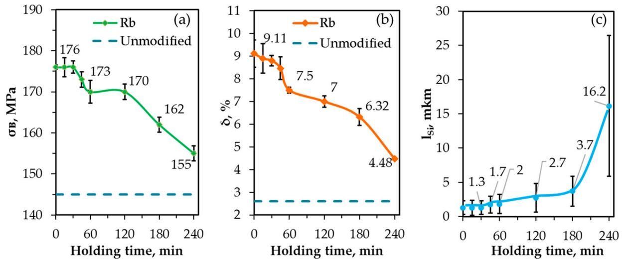
**Figure 7.** Effect of melt holding time after rubidium modification on: (a) ultimate strength; (b) relative elongation; (c) the average length of eutectic silicon particles.
