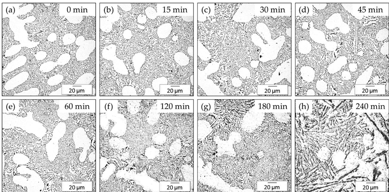
**Figure 8.** Effect of the melt holding time after modification of the microstructure of alloy 3. (a) 0 min.; (b) 15 min.; (c) 30 min.; (d) 45 min.; (e) 60 min.; (f) 120 min.; (g) 180 min.; (h) 240 min.
