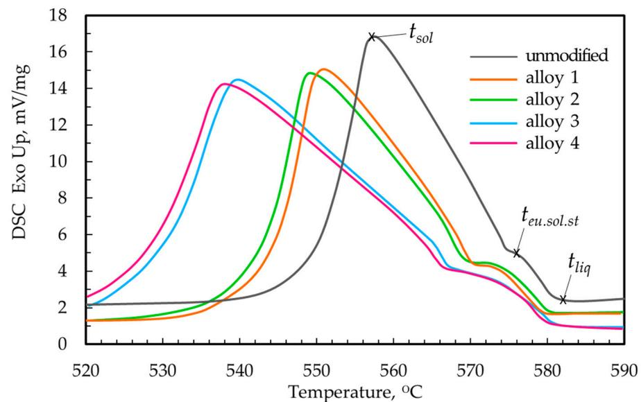
**Figure 4.** Thermograms of experimental alloys.
