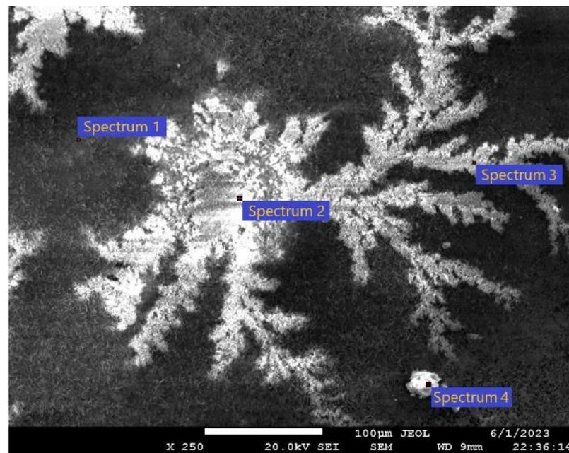
**Figure 10.** SEM-EDS analysis of degradation products of RS-treated Zn-1%Mg-0.1%Ca alloy.
