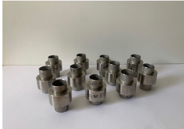
Figure 17. Illustration of crimped joints.
