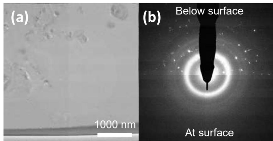
**Figure 8.** (a) A TEM image and (b) diffraction result taken from a FIB lift-out of the surface of the  $\text{Mg}_{64}\text{Cu}_{25}\text{Y}_{11}$  sample. At the very surface of the sample, a distinct lack of features in the image and an amorphous halo was observed. The composition in this spot was measured as  $\text{Mg}_{54}\text{Cu}_{40}\text{Y}_6$ .
