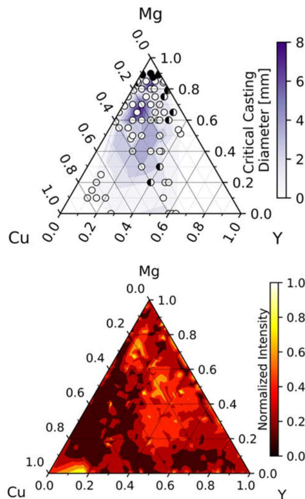
**Figure 5.** (Top) a contour map of critical casting diameter (mm) overlaid with a scatterplot showing the experimental literature results for glass-forming ability [61–68] for the given compositions: (○) amorphous, (◐) partly amorphous, and (●) crystalline. (Bottom) the normalized optical intensity of the printed beads with total saturation of the camera at 1 and no reflected light at 0. The data are plotted for the nominal composition.
