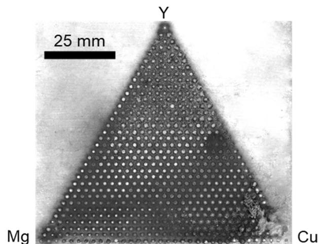
**Figure 4.** An optical image of a printed Mg-Cu-Y composition library taken with a high-contrast background and diffuse lighting. The nominal compositions of each bead range from 0–100 at% with 3 at% intervals in all three elements. This plate was printed using a 330 W laser power and a pulse duration less than 3 s, which varied according to composition. The total volume flowrate was kept constant at 2.4 cm<sup>3</sup> min<sup>-1</sup>.
