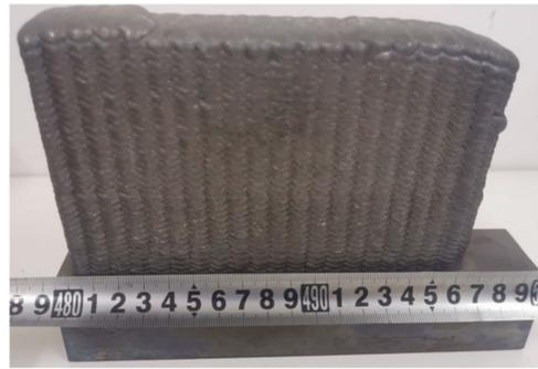
**Figure 1.** WAAM test piece after heat treatment.
