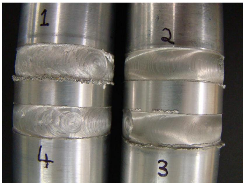
**Figure 15.** Visual inspection of the surfaces obtained from OFSW, reprinted with permission from [22], 2023, Elsevier.
