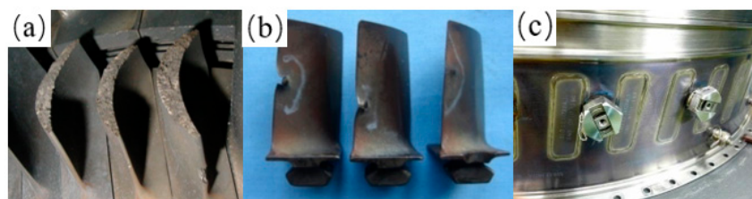
Figure 1. Typical vibration fatigue weak link of aeroengine (a) turbine blades; (b) fan/compressor blades; (c) thin-walled weldments.
