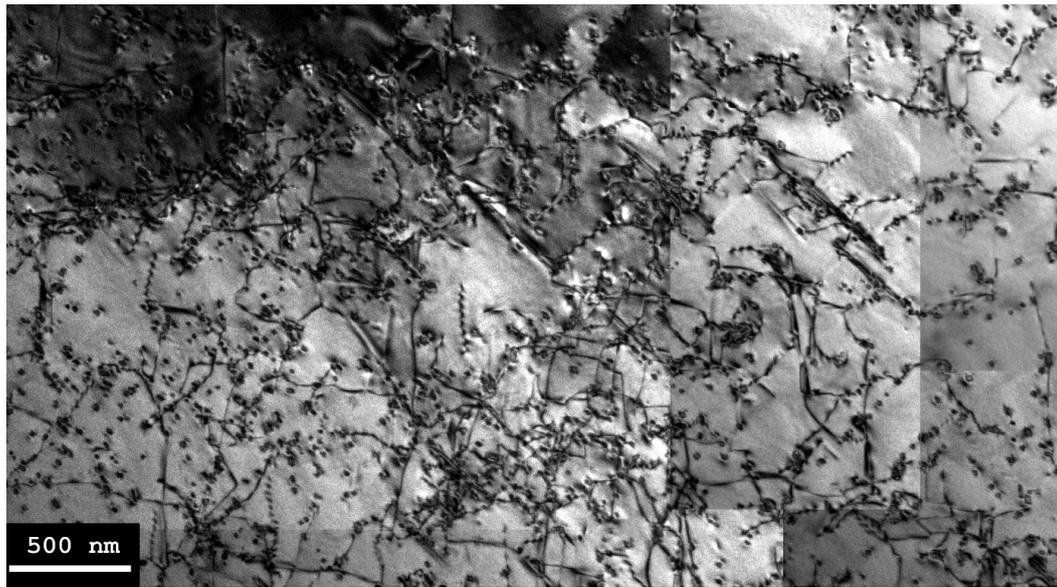
**Figure 8.** Sample stabilized at 800 °C for 10 h. Dislocation substructure of austenitic grain in orientation near the pole [001] with strong reflection type 200. TEM micrograph.
