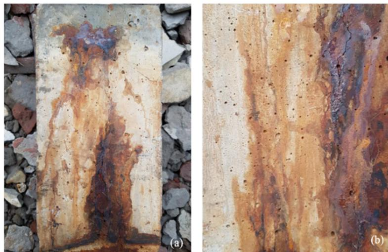
**Figure 7.** (a) Surface pitting on column specimen after 5 days. (b) Surface pitting on column specimen after 8 days.
