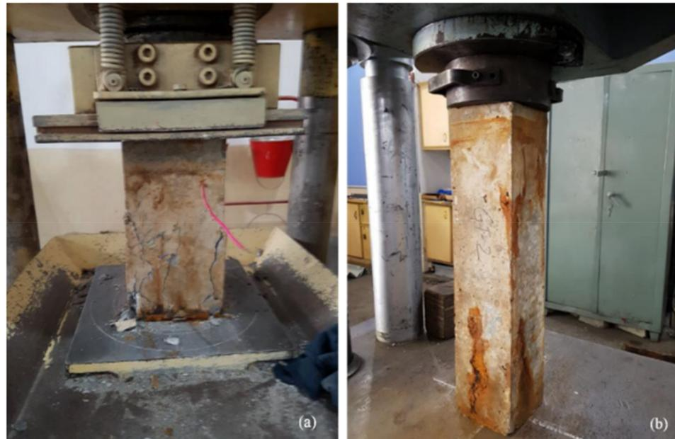
**Figure 8.** (a) Compression test 300 mm specimen. (b) Compression test 700 mm specimen.
