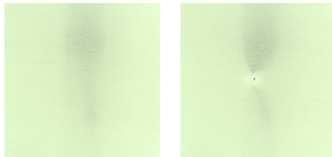
Figure 14. Scratch and bulge defects in the absence of a dark field.
