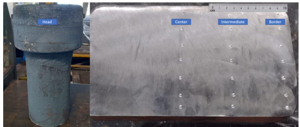
Figure 9. The markings from the Brinell hardness test.
