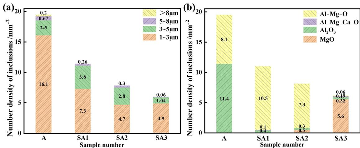
**Figure 7.** Differences between S1 and S3 in the inclusion number density of the molten steel samples: (a) different inclusion sizes and (b) inclusion types.
