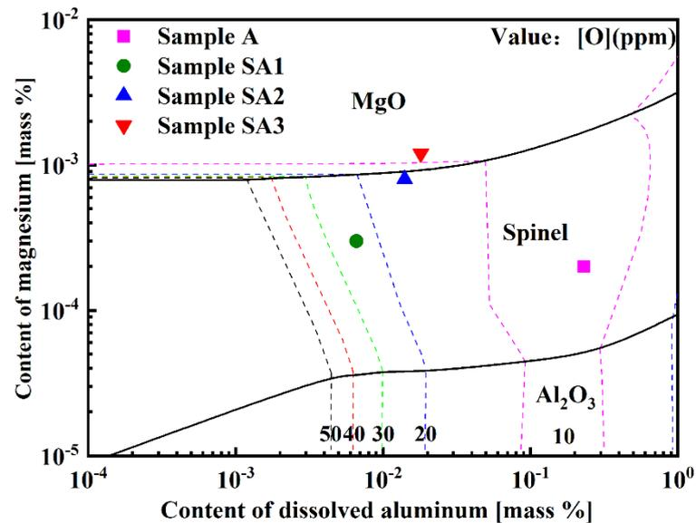
Figure 13. Al-Mg stable phase diagram of 15-5PH stainless steel at 1600 °C.
