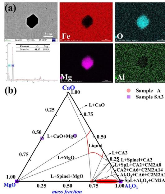
**Figure 6.** Morphology and makeup of the typical inclusions in Sample A3: (a) elemental distribution of the point inclusions and (b) composition distributions of the inclusions in Samples A and A3 in the MgO-Al<sub>2</sub>O<sub>3</sub>-CaO phase diagram. At 1600 °C, the solid lines depict the boundaries between several phases.
