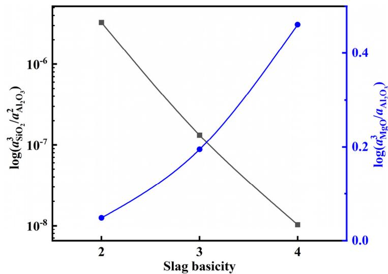
Figure 12. Dependence of  $\log(a_{SiO_2}^3/a_{Al_2O_3}^2)$  and  $\log(a_{MgO}^3/a_{Al_2O_3})$  on slag basicity.
