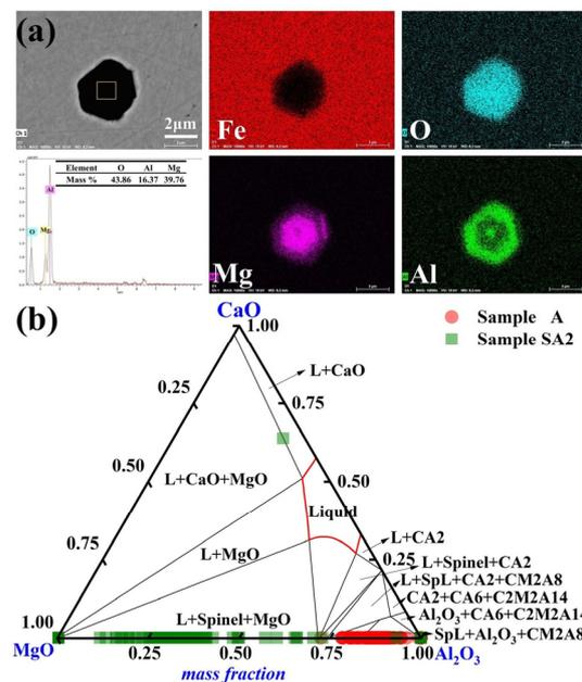
**Figure 5.** Common inclusions in Sample A2 had the following morphology and composition: (a) elemental distribution of the point inclusions and (b) composition distributions of the inclusions in Samples A and A2 in the MgO-Al<sub>2</sub>O<sub>3</sub>-CaO phase diagram. At 1600 °C, the solid lines depict the boundaries between several phases.
