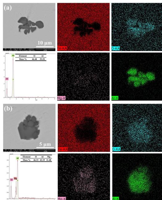
**Figure 3.** Typical inclusion morphology and makeup of Sample A: (a)  $\text{Al}_2\text{O}_3$  inclusion; (b)  $\text{Al}_2\text{O}_3 \cdot \text{MgO}$  inclusion.
