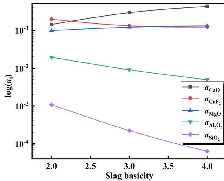
Figure 11. Relationship of activity with slag basicity.
