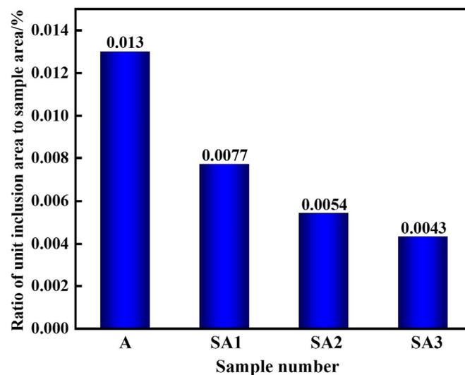
**Figure 8.** Ratio of unit inclusion area to sample-scanning area in various samples after slag reaction.
