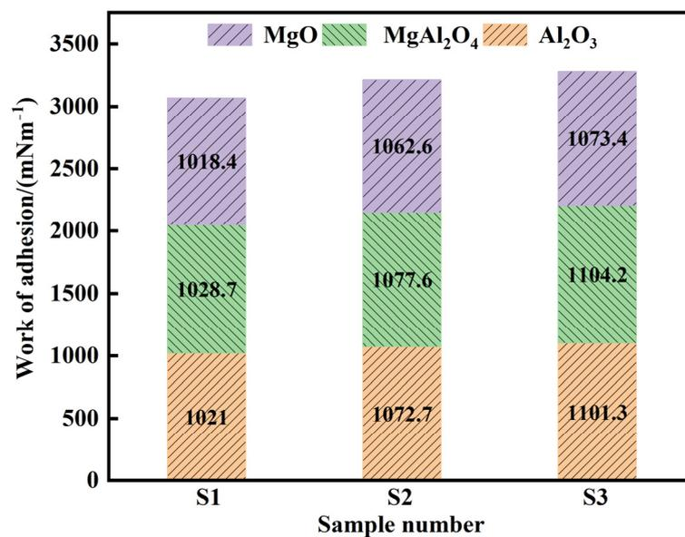
**Figure 10.** Adhesion work between the Al<sub>2</sub>O<sub>3</sub>, MgAl<sub>2</sub>O<sub>4</sub>, and MgO inclusions in various refining slags.
