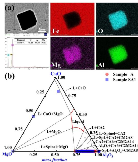
**Figure 4.** Common inclusions in Sample A1 had the following morphology and composition: (a) elemental distribution of the point inclusions and (b) composition distributions of the inclusions in Samples A and A1 in the MgO-Al<sub>2</sub>O<sub>3</sub>-CaO phase diagram. At 1600 °C, the solid lines depict the boundaries between several phases.
