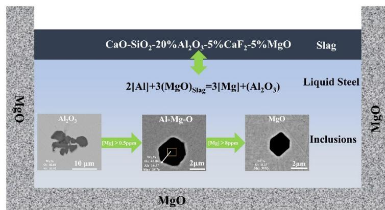
Figure 14. The CaO-MgO-SiO<sub>2</sub>-Al<sub>2</sub>O<sub>3</sub>-CaF<sub>2</sub> slag and inclusion reaction evolution mechanism in 15-5PH stainless steel.
