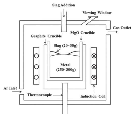
**Figure 1.** Diagram of the testing equipment.
