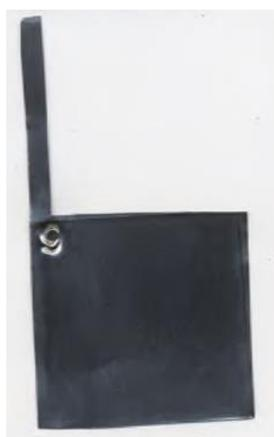
**Figure 1.** Photograph of a metal sample for electrochemical testing.
