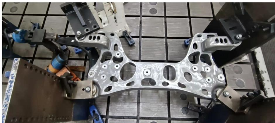
**Figure 27.** Lateral force fatigue endurance test of aluminium alloy front subframe on bench.
