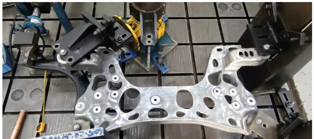
**Figure 26.** Longitudinal fatigue endurance test of aluminium alloy front subframe on bench.
