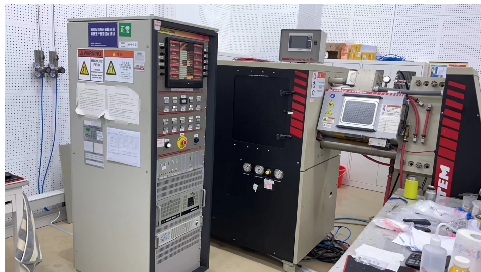
Figure 3. Gleeble-3500 testing machine.
