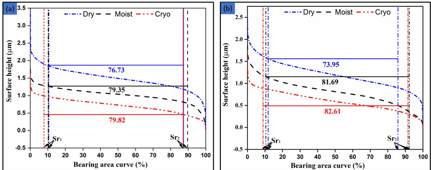
**Figure 10.** Surface height variation of finished (a) AM and (b) conventional samples at a DOC of 40  $\mu\text{m}$  and table feed of 13 m/min in dry, moist, and cryogenic conditions.
