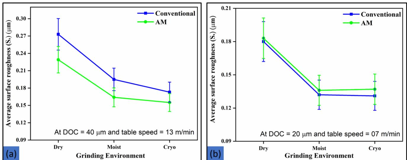
**Figure 8.** Average surface roughness obtained from atomic force microscopy: (a) at a DOC of 40  $\mu\text{m}$  and table feed of 13 m/min and (b) at a DOC of 20  $\mu\text{m}$  and table feed of 07 m/min.
