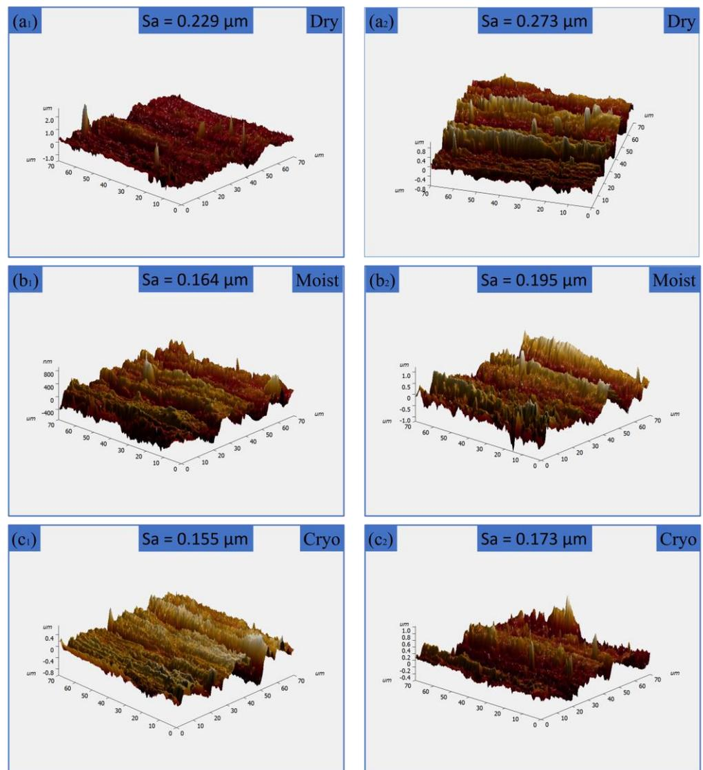
**Figure 9.** AFM images of finished AM and conventionally processed samples at DOC of 40  $\mu\text{m}$  and table feed of 13 m/min: (a<sub>1</sub>) dry for AM, (a<sub>2</sub>) dry for conventional, (b<sub>1</sub>) moist for AM, (b<sub>2</sub>) moist for conventional, (c<sub>1</sub>) cryogenic for AM, and (c<sub>2</sub>) cryogenic for conventional samples.
