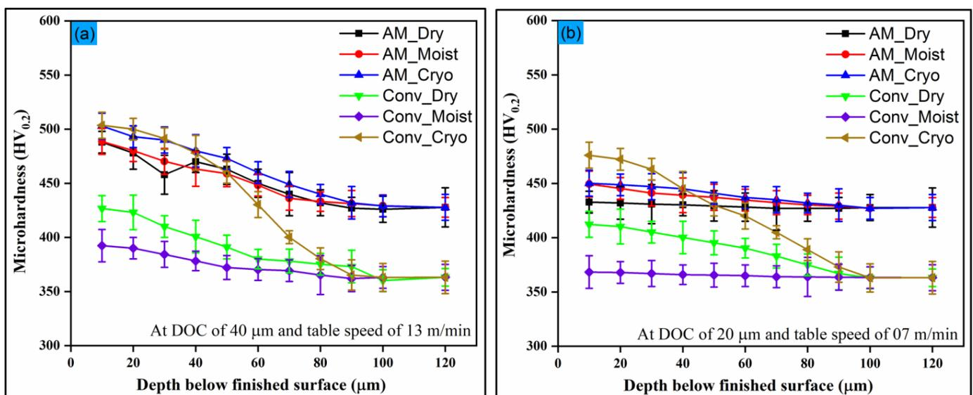
**Figure 12.** Variation in microhardness results for finished DMLS and conventional samples at (a) DOC of 40 μm and table feed of 13 m/min and (b) DOC of 20 μm and table feed of 07 m/min.
