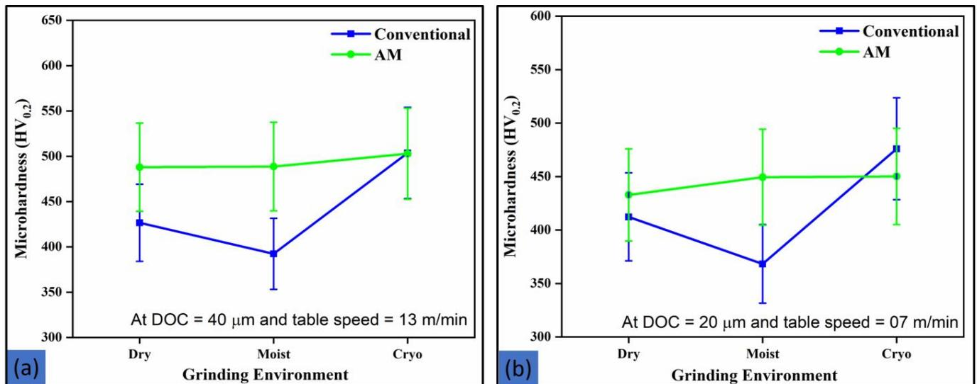
**Figure 11.** Maximum microhardness for AM and conventional components at (a) DOC of 40 μm and table feed of 13 m/min and (b) DOC of 20 μm and table feed of 07 m/min under different grinding conditions.
