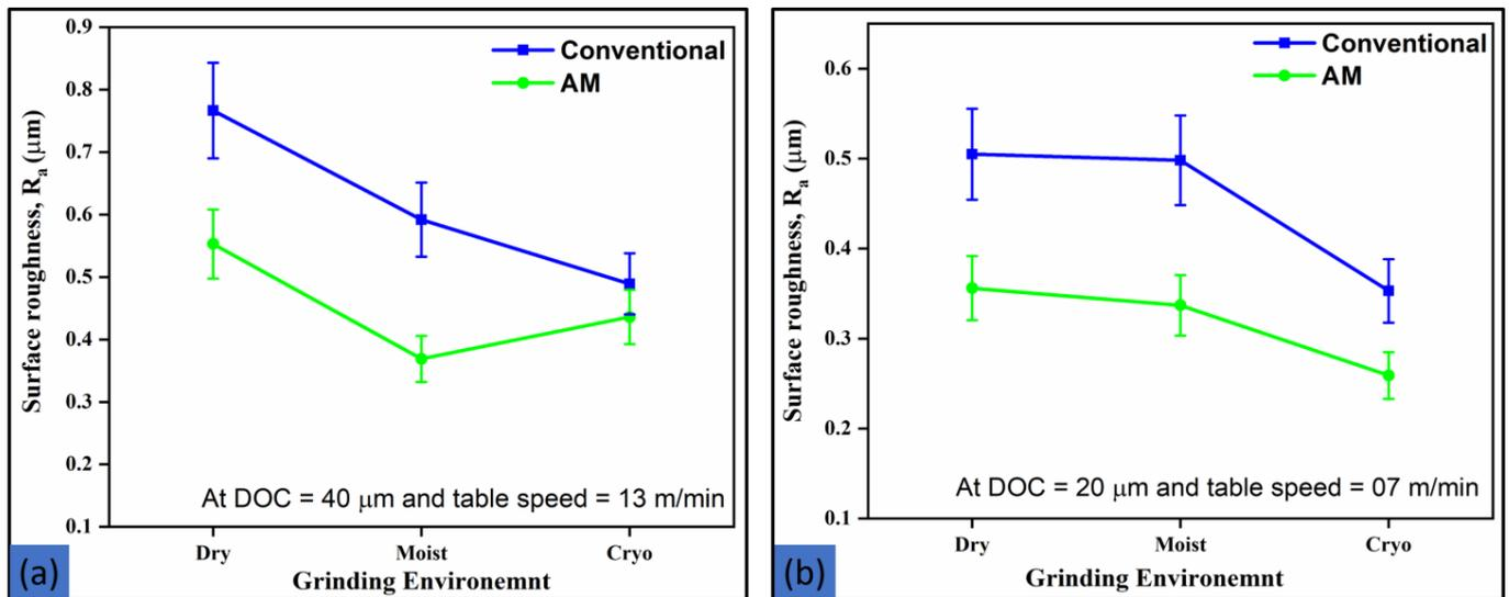
**Figure 6.** Surface roughness of finished AM and conventionally processed components: (a) at DOC of 40  $\mu\text{m}$  and table feed of 13 m/min and (b) at DOC of 20  $\mu\text{m}$  and table feed of 07 m/min.
