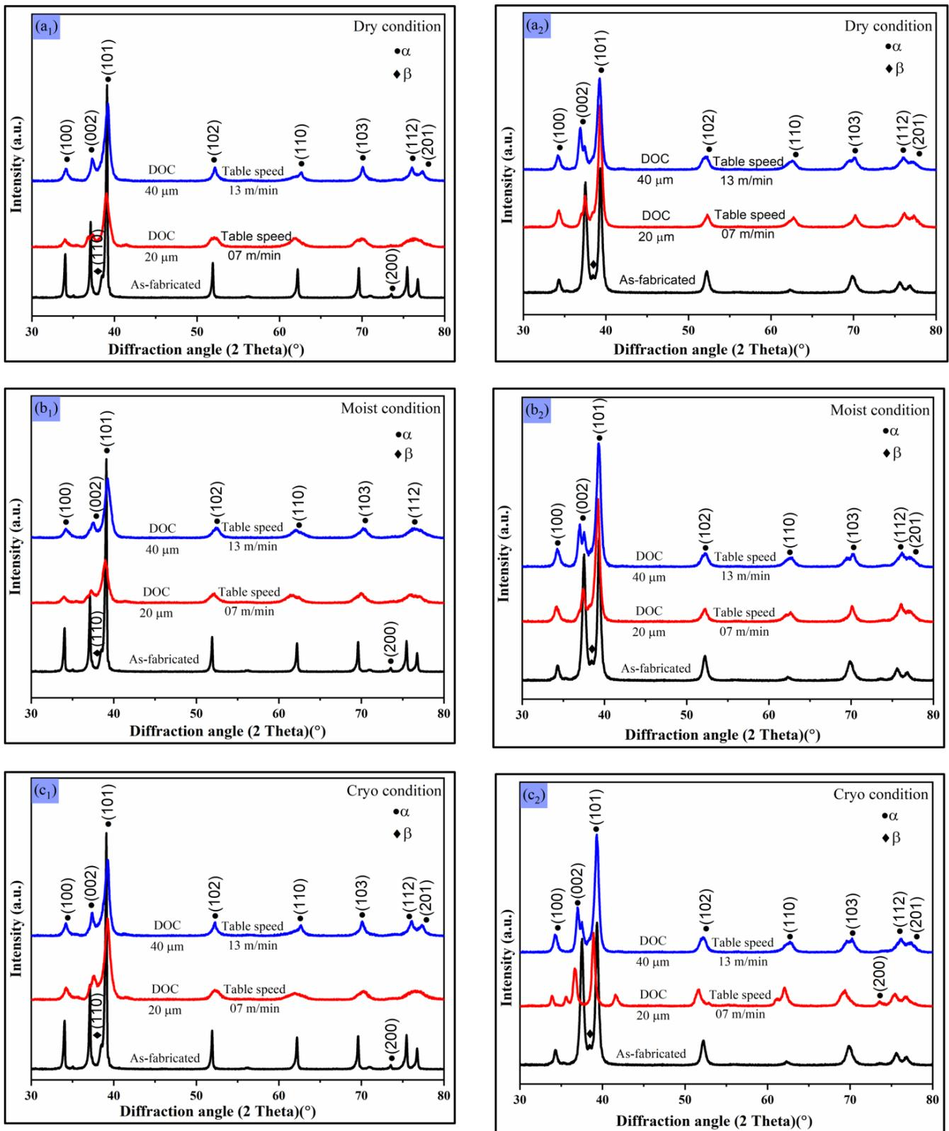
**Figure 13.** XRD patterns at DOC of 40, 20  $\mu\text{m}$  and table feeds of 07, 13 m/min for various grinding conditions: (a<sub>1</sub>) dry for AM, (a<sub>2</sub>) dry for conventional, (b<sub>1</sub>) moist for AM, (b<sub>2</sub>) moist for conventional, (c<sub>1</sub>) cryogenic for AM, and (c<sub>2</sub>) cryogenic for conventional samples.
