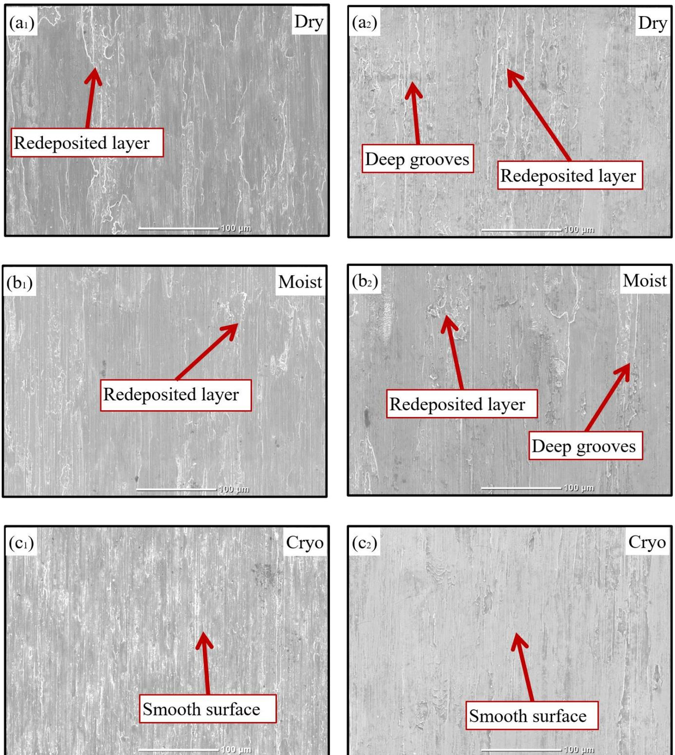
**Figure 7.** SEM images of finished AM and conventionally processed samples at a DOC of 40 μm and table feed of 13 m/min, in: (a<sub>1</sub>) dry for AM, (a<sub>2</sub>) dry for conventional, (b<sub>1</sub>) moist for AM, (b<sub>2</sub>) moist for conventional, (c<sub>1</sub>) cryogenic for AM, and (c<sub>2</sub>) cryogenic for conventional samples.
