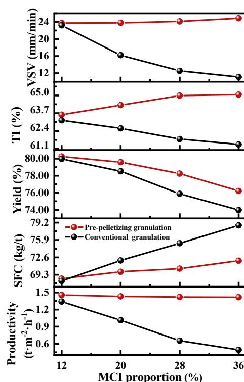
**Figure 5.** Sintering indexes of different MCI proportions using conventional and pre-pelletizing granulation.
