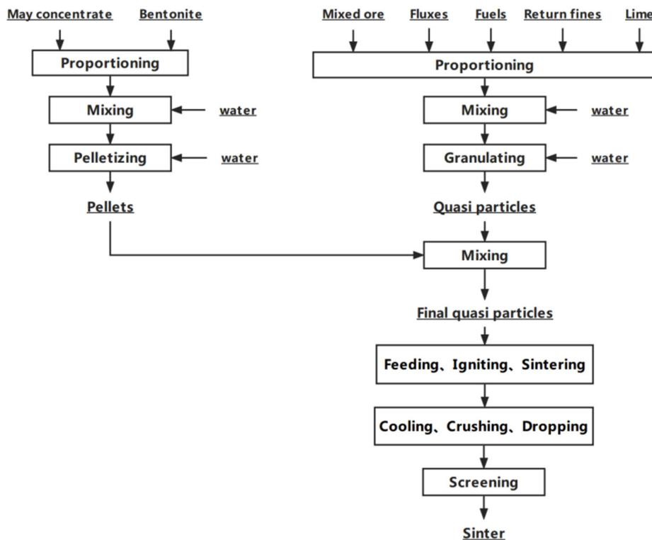
**Figure 2.** The process of pre-pelletizing granulation sintering.
