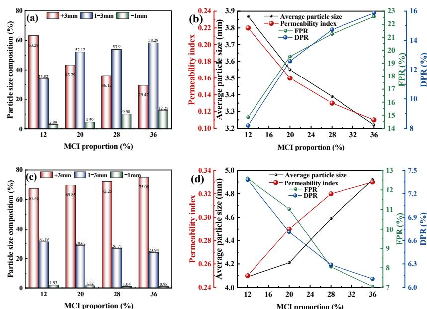
**Figure 3.** Effect of MCI proportion on granulation. Conventional granulation: (a,b); Pre-pelletizing granulation: (c,d).
