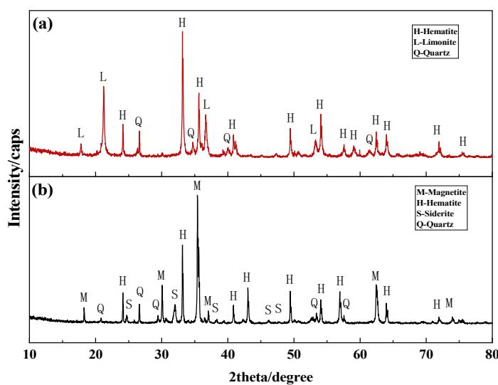
**Figure 1.** XRD pattern of Blended ore (a) and MCI (b).
