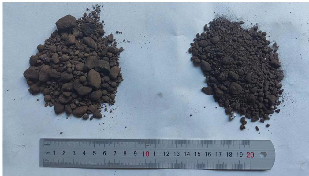
**Figure 4.** The morphology of quasi-particles of conventional granulation (right) and pre-pelletizing granulation (left) at 28% MCI proportion.
