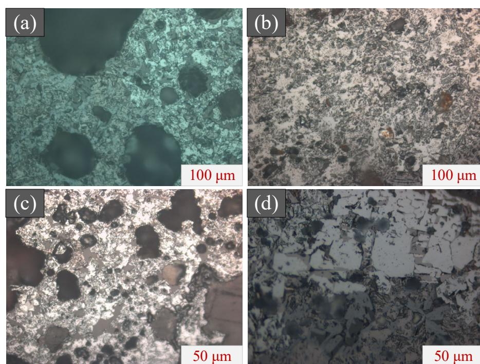
**Figure 6.** Microstructure of finished sinter from conventional and pre-pelletizing granulation sintering at 28% of MCI proportion. (a) conventional granulation sinter; (b) pre-pelletizing granulation sinter; (c) MCI pellet sinter; (d) conventional material and MCI pellet connection.
