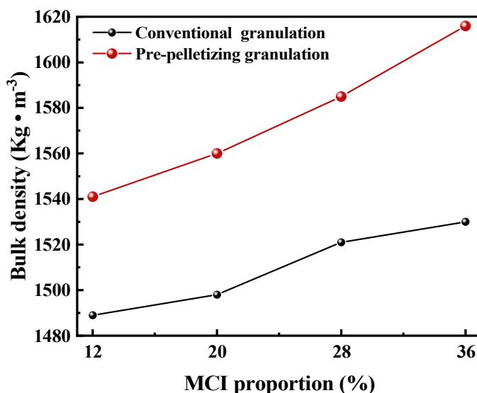
**Figure 8.** Quasi-particles bulk density from conventional and pre-pelletizing granulation.
