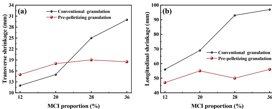
**Figure 7.** Transverse (a) and longitudinal (b) shrinkage of sinter.
