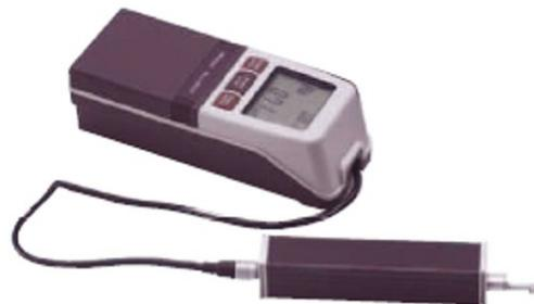
**Figure 5.** Mitutoyo brand SJ 201 surface roughness measuring device.
