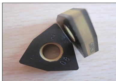
Figure 2. WNMA 080408 IC5005 CVD-coated cutting inserts.
