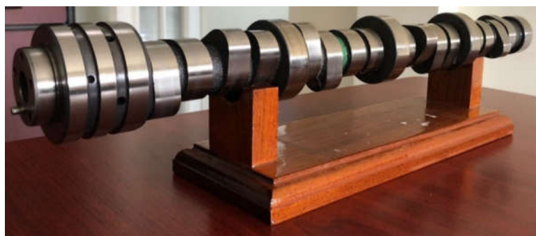
Figure 5. ADI low alloyed with vanadium camshaft 5.7L with 16 intake and exhaust lobes.
