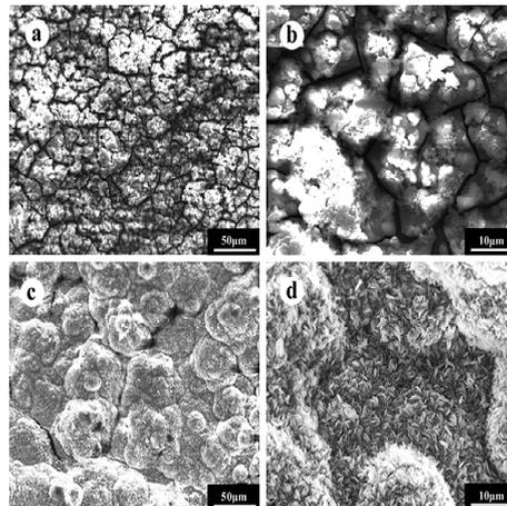
**Figure 8.** The SEM images of the striped surfaces after immersion in Hank's solution for 14 days: (a,b) crystalline Mg65Zn30Ca5; (c,d) amorphous Mg65Zn30Ca5 [40].
