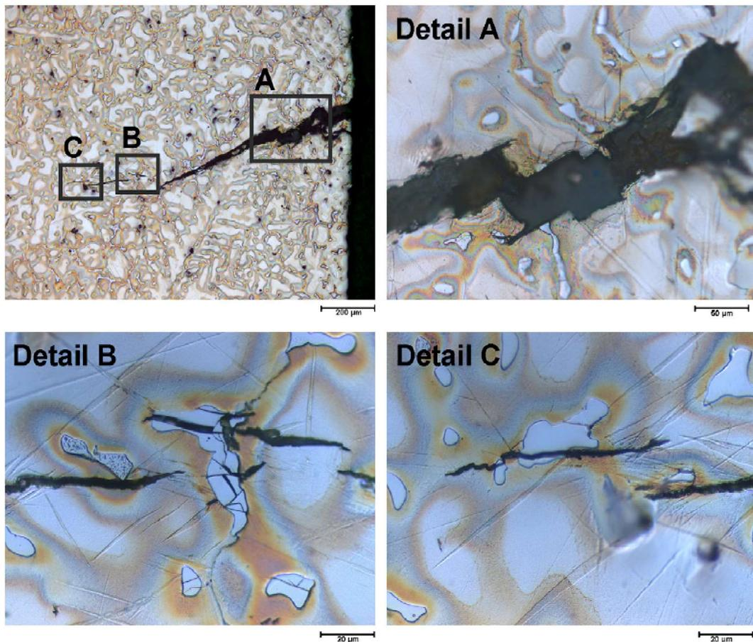
**Figure 7.** The detailed SCC of AZ91 in double-distilled water at a strain rate of  $3 \times 10^{-7} \text{s}^{-1}$ . Adapted with permission from Ref. [37]. Copyright 2008, Elsevier.
