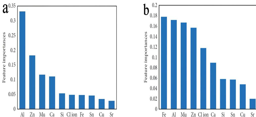
**Figure 6.** The importance of input features for corrosion potential (a) and corrosion current (b) prediction models [26].
