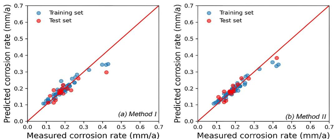
**Figure 17.** The prediction accuracy of corrosion rate prediction models based on input features derived from feature generation method I and feature generation method II. Adapted with permission from Ref. [56]. Copyright 2021, Elsevier.
