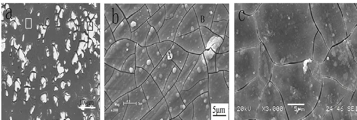
**Figure 10.** The corrosion morphology of magnesium alloys in simulated physiological environments: (a) AZ91 magnesium alloy exposed to c-SBF for 1 day; (b) Mg-Mn-Zn alloy exposed to Hanks' solution for 12 days; (c) pure magnesium after 30 days of exposed to c-SBF. Adapted with permission from Ref. [41]. Copyright 2011, Elsevier.
