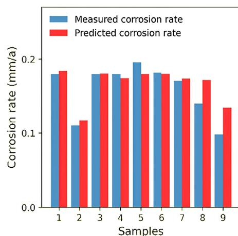
**Figure 18.** The comparison between the corrosion rates measured through immersion experiments and the corrosion rates predicted by the machine learning model. Adapted with permission from Ref. [56]. Copyright 2021, Elsevier.
