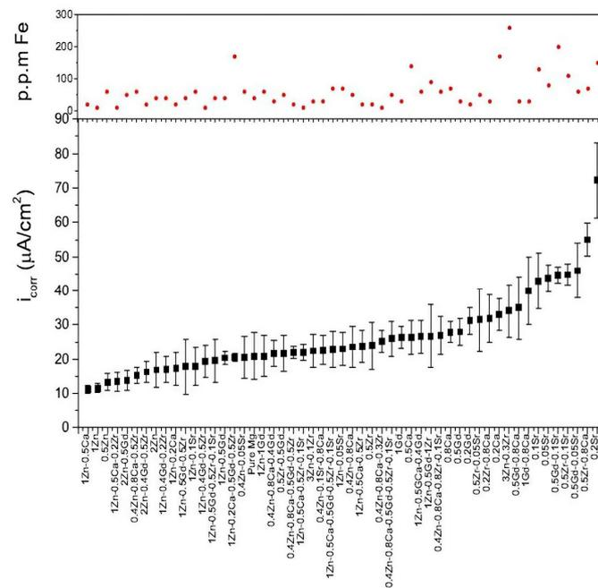
Figure 1. Corrosion rate in terms of corrosion current density ( $i_{corr}$ ). Adapted with permission from Ref. [21]. Copyright 2016, Elsevier.
