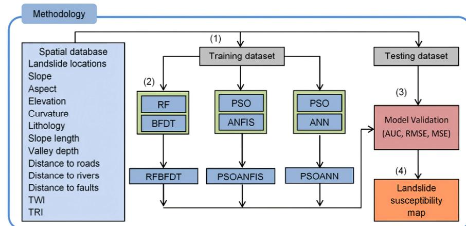
Figure 21. The method flowchart [65].
