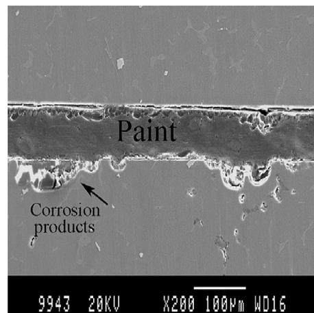
**Figure 11.** The cross-sectional image of AZ91 magnesium alloy exposed to c-SBF. Adapted with permission from Ref. [41]. Copyright 2011, Elsevier.
