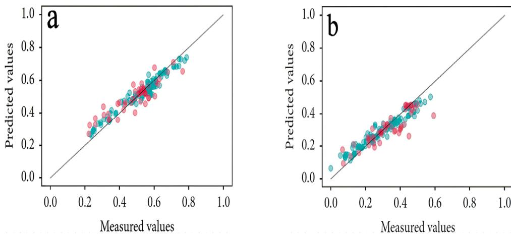
**Figure 5.** The prediction results of the corrosion potential and current density corresponding to the RF algorithm. (a) The corrosion potential prediction results of the RF algorithm. (b) The algorithm's predictions for the current corrosion [26].
