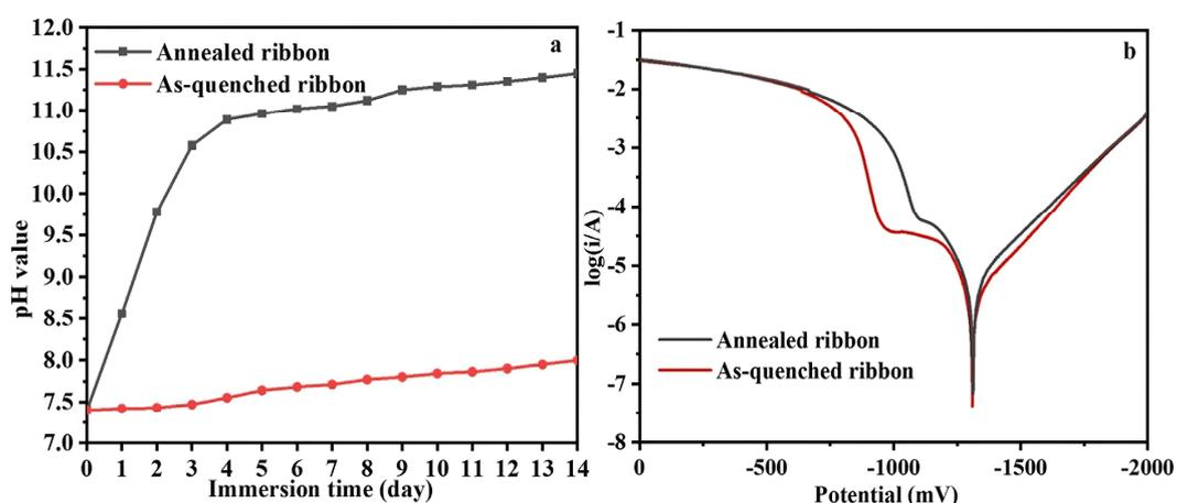
**Figure 9.** (a) The variation in pH of the Hank's solution containing quenched/annealed thin strips, and (b) the typical polarization curves of the quenched and annealed strips [40].
