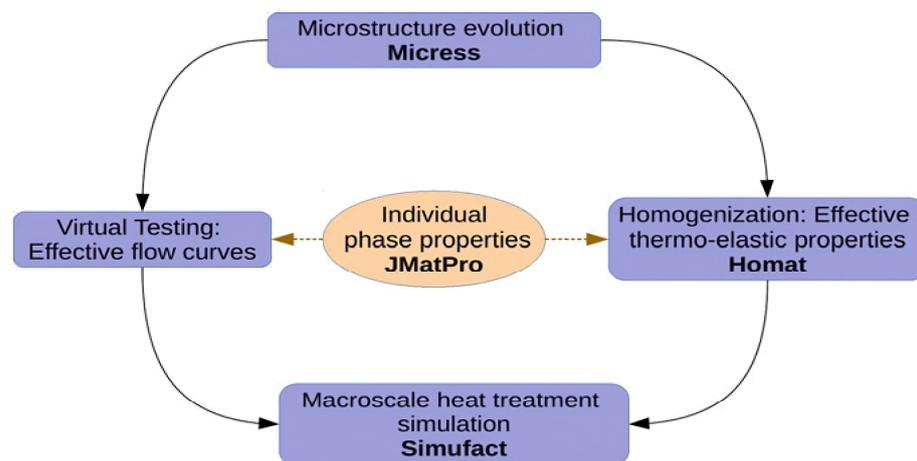
**Figure 20.** The multiscale simulation workflow. Adapted with permission from Ref. [64]. Copyright 2023, AIP Publishing.
