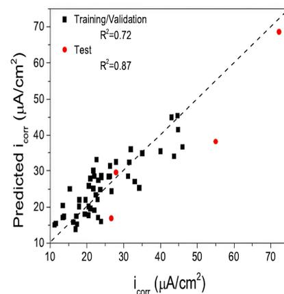
Figure 2. Correlation between predicted  $i_{corr}$  and observed  $i_{corr}$ . Adapted with permission from Ref. [21]. Copyright 2016, Elsevier.
