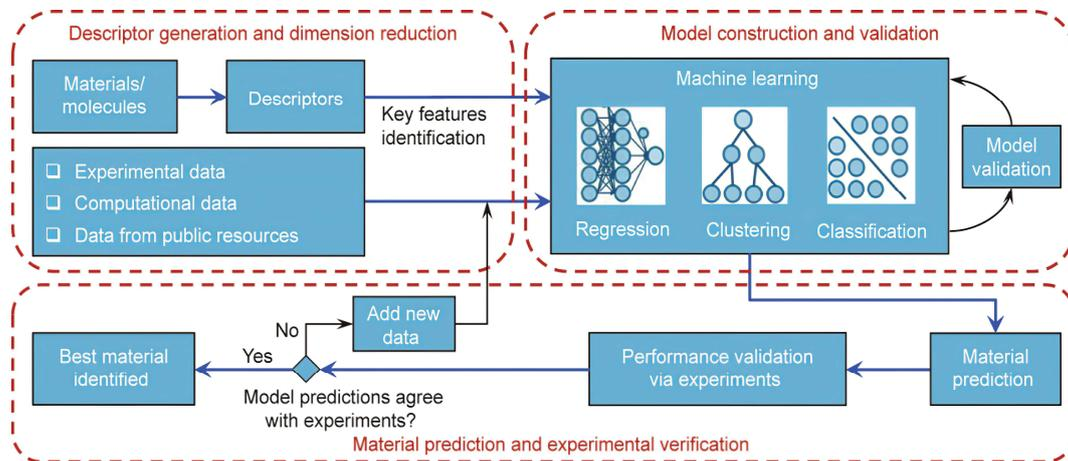
**Figure 19.** The general workflow of material discovery and design based on machine learning [61].
