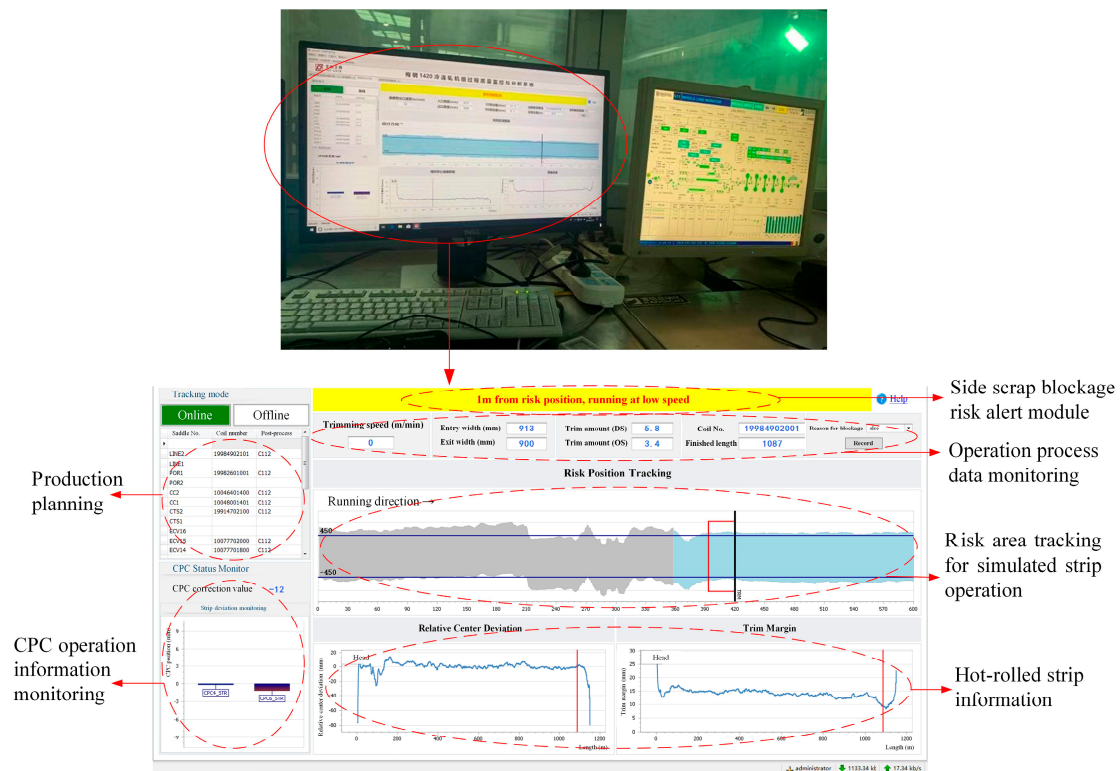
Figure 16. Interface of the side scrap blockage pre-control model.
