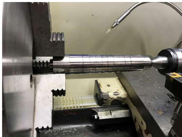
**Figure 2.** General view of a Ti-6Al-4V alloy workpiece with different regime zones in the lathe.
