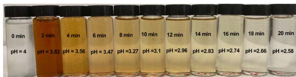
Figure 3. The colour change of the solution as a function of pH at different time intervals ( \text{SO}_2/\text{air} ratio = 0.03, air flow rate = (500 \pm 10) mL min -1 , \text{SO}_2 flow rate = (15 \pm 2) mL min -1 , T = (80 \pm 0.5) °C, agitation speed = 2000 rpm, initial [\text{Mn}] \approx 1 g L -1 ).
