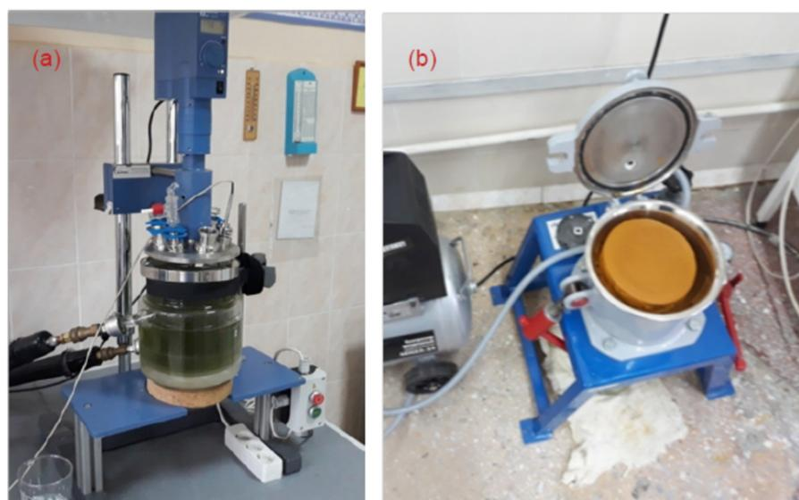
**Figure 3.** General view of the LR-2.ST type reactor (a) and the druk-filter (b).
