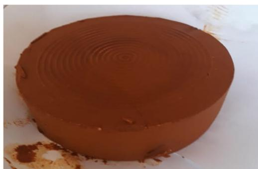
Figure 13. Precipitate obtained after Fe(III) precipitation from direct electrooxidation solutions.
