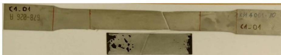
Figure 3. Tensile test on steel + CFRP specimen.
