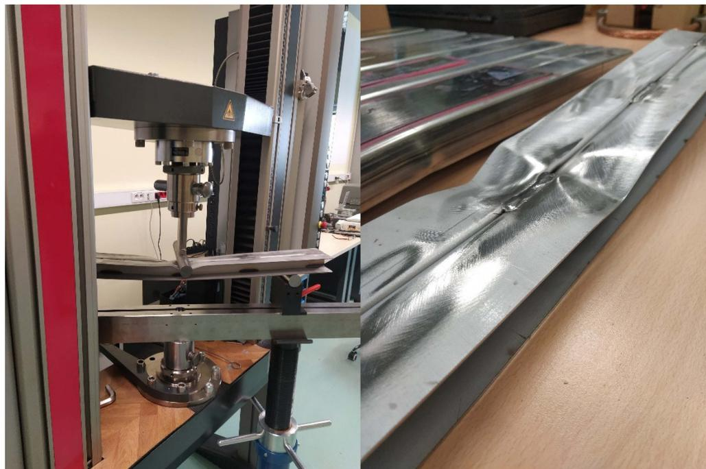
**Figure 1.** Three-point bending test of a steel section reinforced with CFRP tape.
