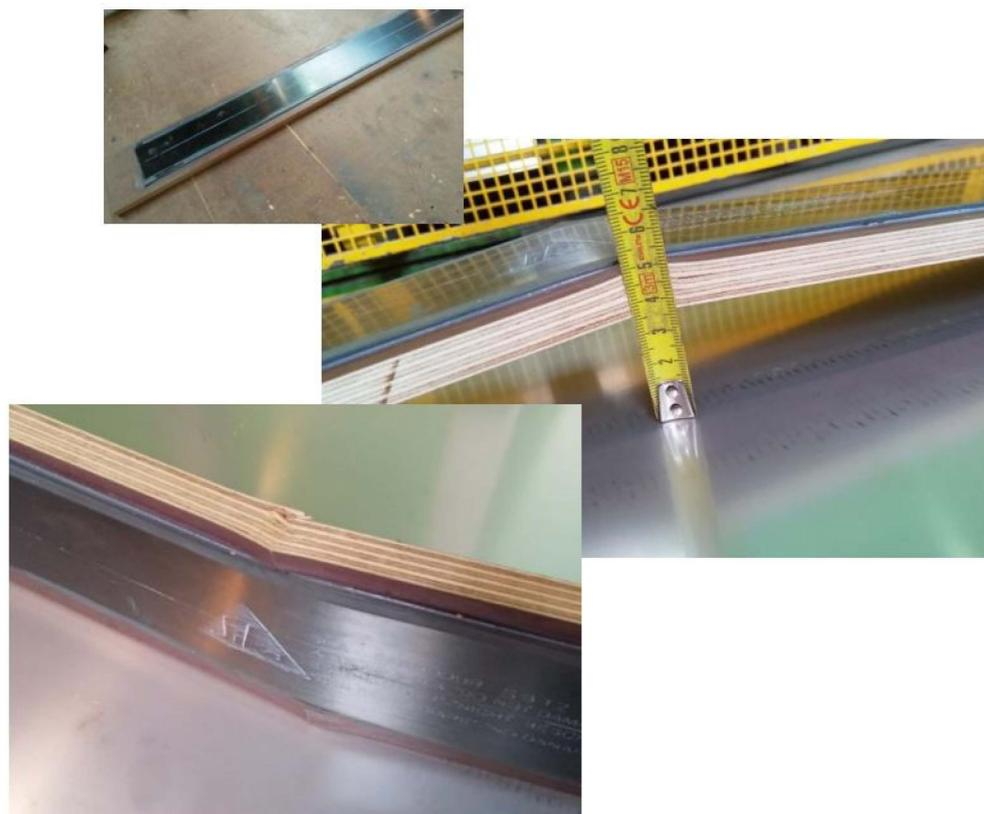
**Figure 5.** Element made of wood-based material reinforced with CFRP subjected to three-point bending.
