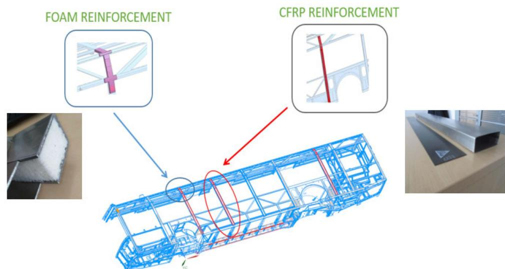
**Figure 7.** Using CFRP tape and foam to reinforce a motor vehicle.
