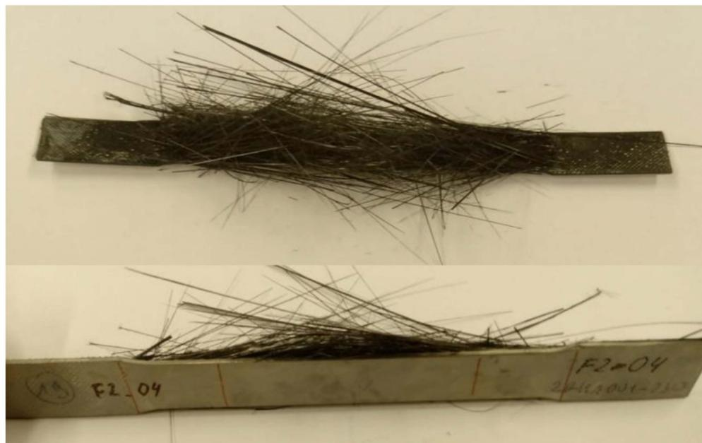
**Figure 4.** Tensile test—steel-CFRP connection.
