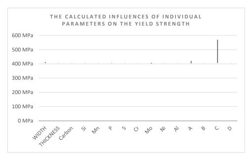
**Figure 8.** The calculated influences of individual parameters on the yield strength while separately changing individual parameter within the individual parameter range.
