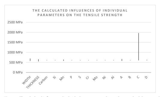
**Figure 7.** The calculated influences of individual parameters on the tensile strength while separately changing individual parameter within the individual parameter range.
