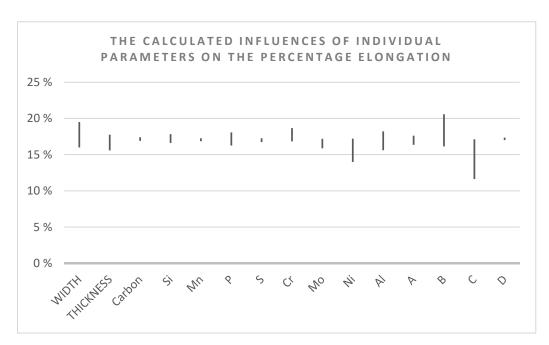
**Figure 4.** The calculated influences of individual parameters on the percentage elongation while separately changing individual parameter within the individual parameter range.
