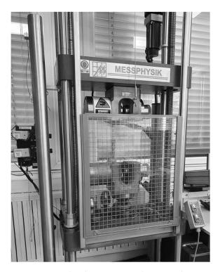
Figure 1. Messphysik Beta 300 tensile test machine.
