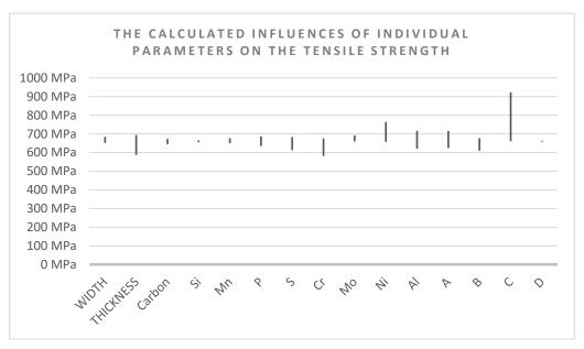
**Figure 2.** The calculated influences of individual parameters on the tensile strength while separately changing individual parameter within the individual parameter range.
