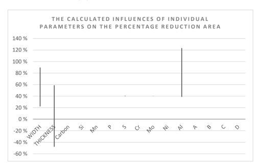
**Figure 10.** The calculated influences of individual parameters on the percentage reduction area while separately changing individual parameter within the individual parameter range.
