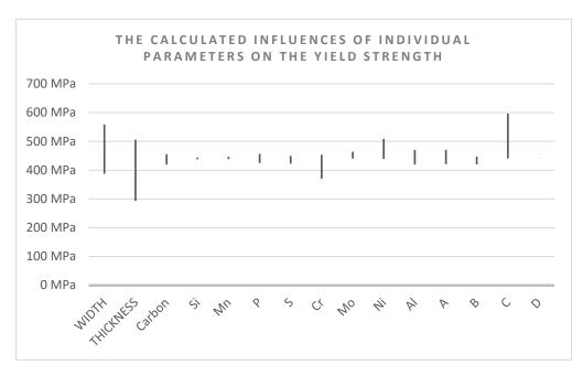
**Figure 3.** The calculated influences of individual parameters on the yield strength while separately changing individual parameter within the individual parameter range.
