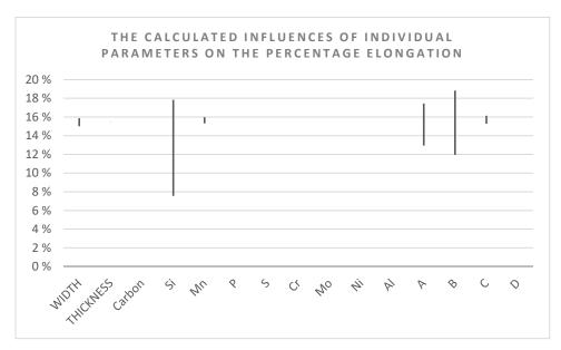
**Figure 9.** The calculated influences of individual parameters on the percentage elongation while separately changing individual parameter within the individual parameter range.
