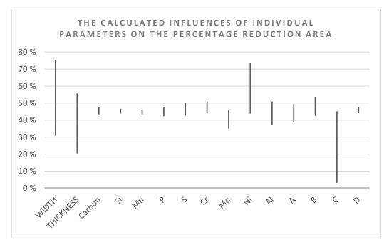
**Figure 5.** The calculated influences of individual parameters on the percentage reduction area while separately changing individual parameter within the individual parameter range.
