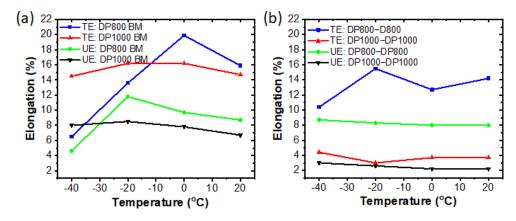
**Figure 9.** Elongation as a function of deformation temperatures for (**a**) DP800 and DP1000 BMs, (**b**) welded DP800 and DP1000 joints, at different deformation temperatures from 20 °C to -40 °C.
