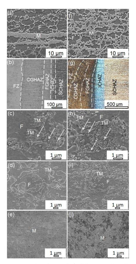
**Figure 3.** SEM and optical micrographs of welded DP800 joint: (**a**) BM; (**b**) Overview of HAZ; (**c**) SCHAZ; (**d**) ICHAZ; (**e**) FZ; and welded DP1000 joint: (**f**) BM; (**g**) Overview of HAZ; (**h**) SCHAZ; (**i**) ICHAZ; (**j**) FZ.
