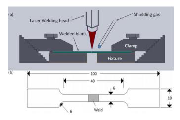
**Figure 1.** Illustrative schematics of (**a**) welding setup, and (**b**) ASTM E8 tensile sample geometry for Quasi-Static Tests (Dimensions are in mm).
