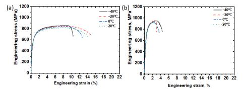
**Figure 6.** Engineering stress–strain curves of (**a**) DP800- and (**b**) DP1000-welded joints at different deformation temperatures.
