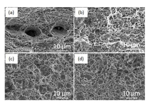
**Figure 12.** Representative SEM images of tensile fracture surfaces of the DP800-welded joints tested at deformation temperature of (a) -40 °C (b) 0 °C; DP1000-welded joints tested at deformation temperature of (c) -40 °C, and (d) 0 °C.
