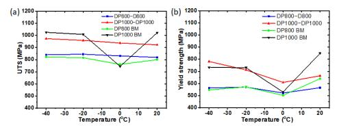
**Figure 7.** (a) UTS and (b) YS of base metals and welded DP steels at different deformation temperatures from -40 °C to 20 °C.
