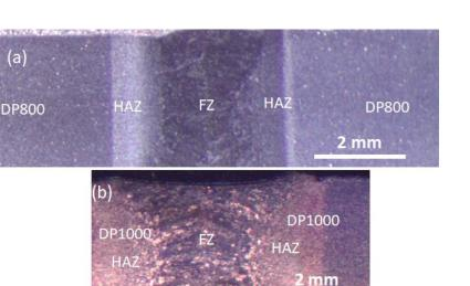
**Figure 2.** (**a**,**b**) light optical micrographs of the cross-sections of the DP800-DP800 and DP1000-DP100 welded joints.
