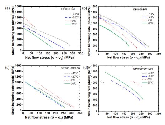
**Figure 11.** Strain hardening rate as a function of net flow stress for (**a**) DP800, (**b**) DP1000 BM, (**c**) DP800 welds, and (**d**) DP1000 welds, at different deformation temperatures from 20 °C to -40 °C.
