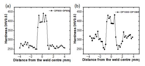
Figure 4. Microhardness profile of the laser-welded (a) DP800-welded joint and (b) D1000-welded joint.
