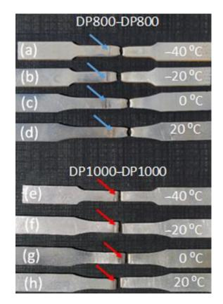
**Figure 8.** Representative fracture samples of DP800-DP800 (**a**–**d**) and DP1000-DP1000 (**e**–**h**) between testing temperatures of -40 °C and 20 °C.
