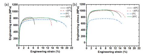
**Figure 5.** Engineering stress-strain curves of (**a**) DP800 and (**b**) DP1000 BM at different deformation temperatures of -40 °C. to 20 °C.
