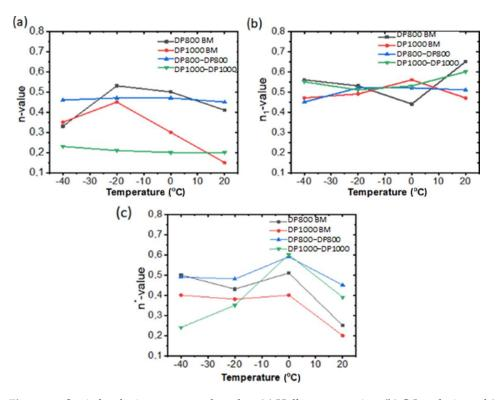
**Figure 10.** Strain hardening exponents based on (**a**) Hollomon equation, (**b**) C-J analysis, and (**c**) equation proposed by Afrin et al. [76] determined at different deformation temperatures for the base metals and welded joints.
