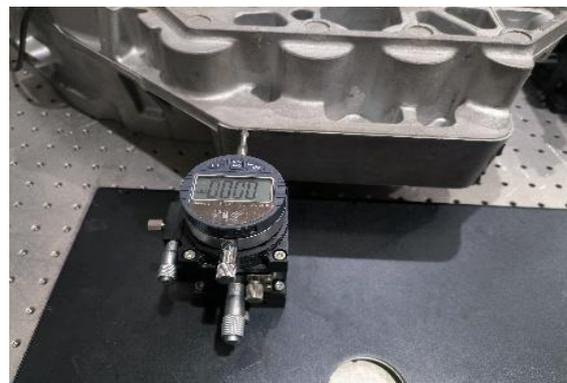
**Figure 14.** Allowance height measurement after machining.
