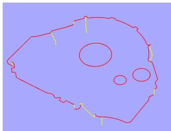
**Figure 12.** Robotic milling path of the flywheel shell in experiment.
