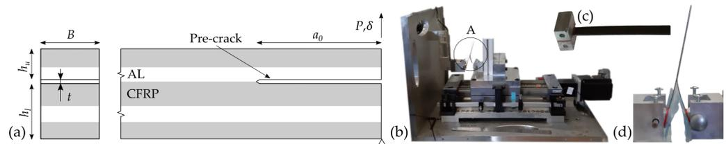
**Figure 2.** Experimental details of delamination fracture energy evaluation procedure: (a) Scheme of ADCB specimens loading, showing pre-crack location. (b) Fracture testing machine equipped with load cell. (c) ADCB specimen with bonded aluminium blocks on both upper and lower arms. (d) Detail A of Figure 2b, showing ADCB specimen with aluminium blocks assembled to testing machine.
