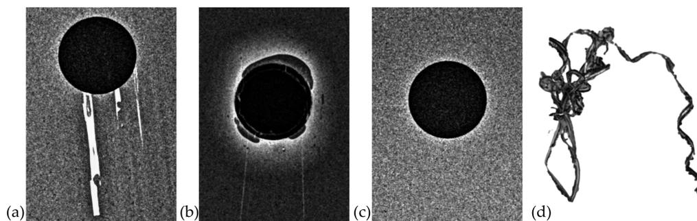
**Figure 5.** X-ray images of representative delamination defects on drilled holes using: (a) CNV drill geometry and (b) CBR drill geometry. (c) Example of delamination-free drilled hole using 2PA drill geometry. (d) Typical chip morphology obtained from drilling operations of FML, regardless of the employed drill.
