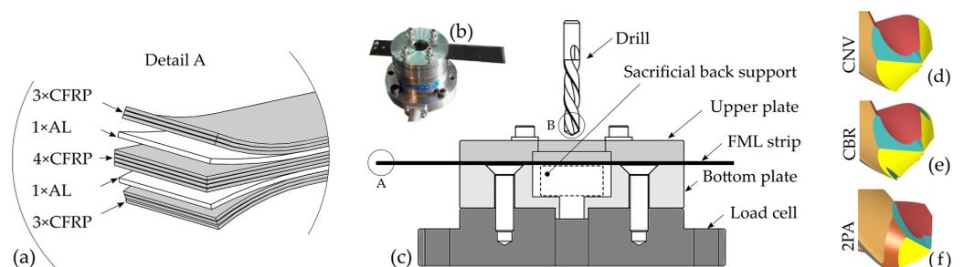
**Figure 1.** Experimental setup used in drilling operations: (a) Fibre metal laminate sequence and layer number of CFRP plies and AA sheets; (b) Clamping system and load cell assemblage with mounted FML strip; (c) Cross-sectional view scheme showing internal placement of back support; Drill tip geometry (detail B in Figure 1c) of conventional drill (d), chip-breaking drill (e) and double-point angle drill (f).
