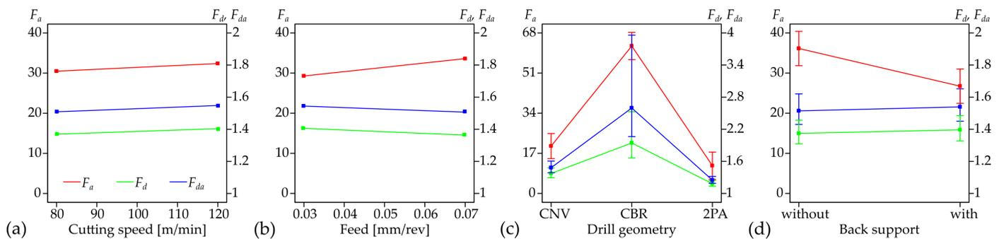
**Figure 6.** ANOVA results on delamination factors in function of: (a) Cutting speed. (b) Feed. (c) Drill geometry. (d) Back support.
