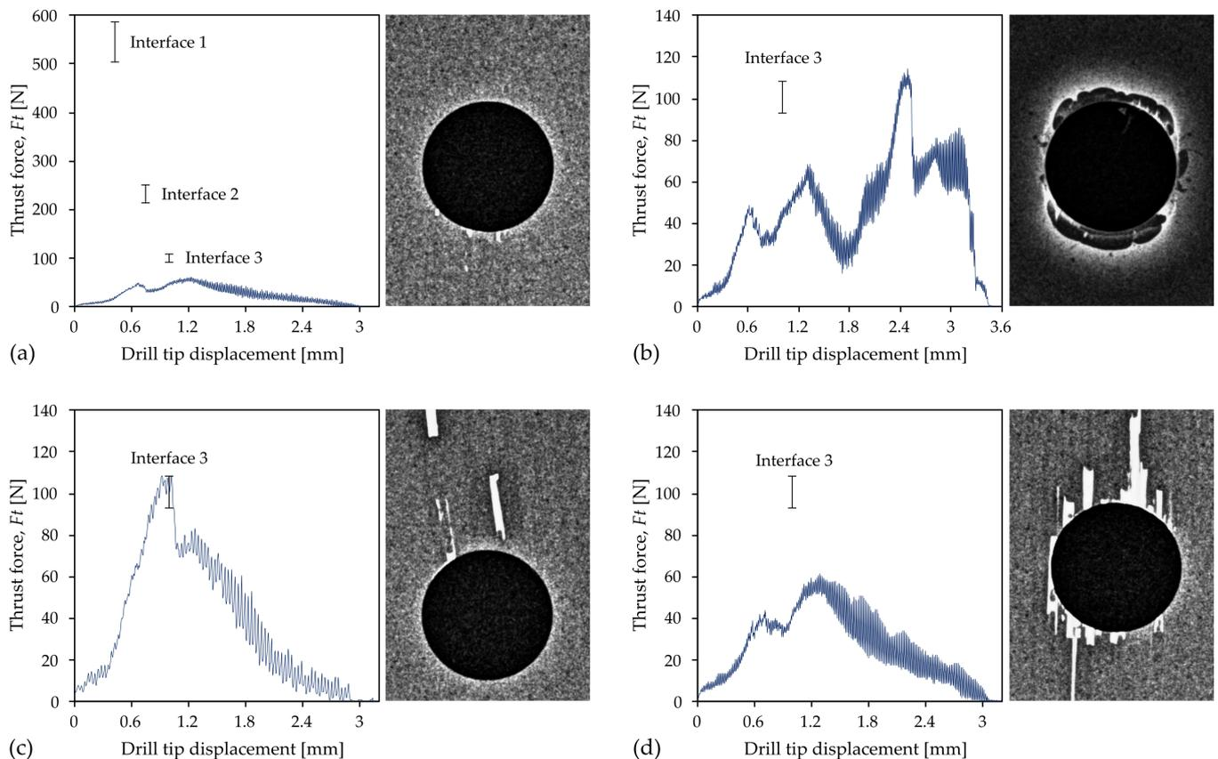
**Figure 9.** Comparison between load–tool displacement curves, calculated critical load and X-ray images of drilled hole for: (a) CNV drill at 120 m/min and 0.03 mm/rev; (b) CNV drill at 100 m/min and 0.07 mm/rev; (c) CBR drill at 120 m/min and 0.03 mm/rev; (d) CNV drill at 80 m/min and 0.03 mm/rev.
