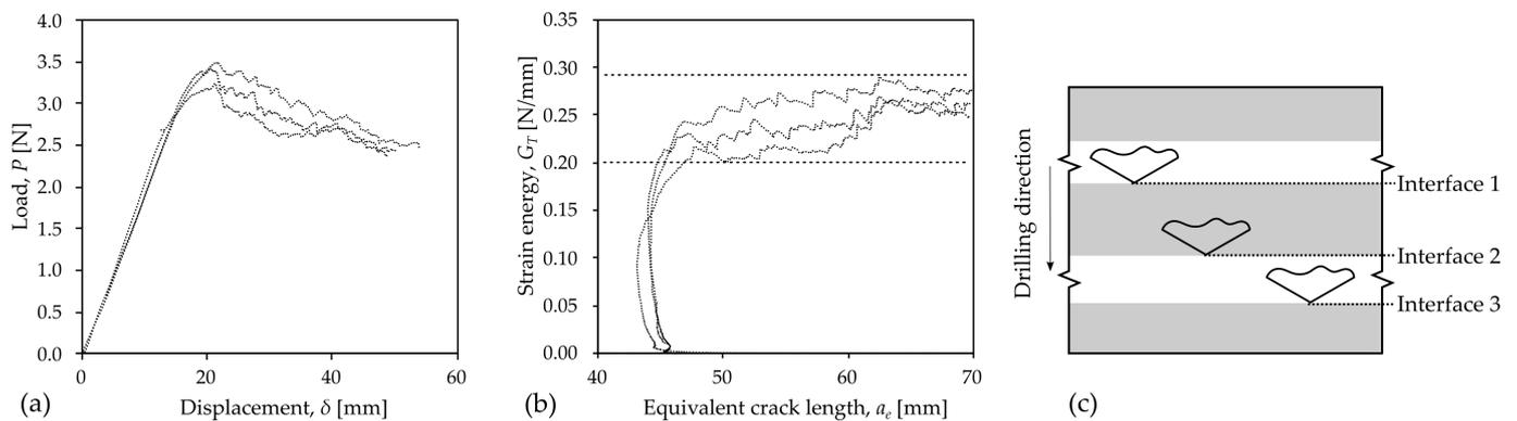
**Figure 8.** Load–displacement and energy release rate results obtained from ADCB fracture tests: (a) Load–displacement curves. (b) Resistance curves; (c) Interfaces where delamination occurrence has been analysed.
