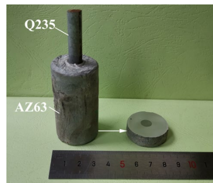
Figure 1. The sample obtained by composite casting.
