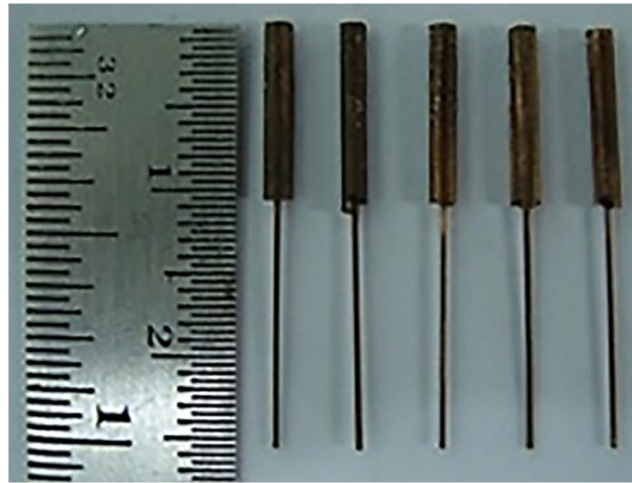
Figure 9. WTET fabricated high-aspect-ratio micro-pins (Reprinted/Adapted with permission from [43]. 2020, Elsevier. ©).
