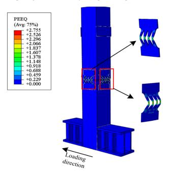
Figure 4. PEEQ (equivalent plastic strain nephogram) of CFST pier and energy dissipator.
