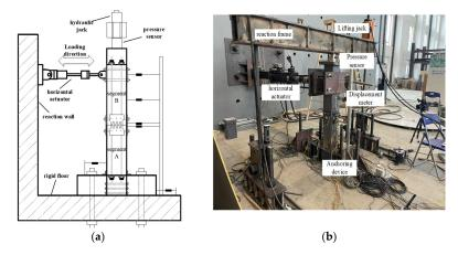
**Figure 8.** Schematic layout of loading and testing apparatus for the proposed static test, (**a**) Schematic diagram of loading device, (**b**) Test loading device diagram.
