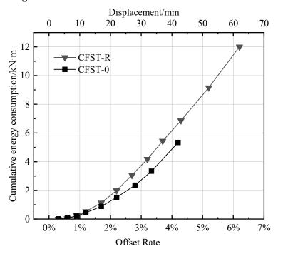
Figure 17. Cumulative energy consumption capacity.
