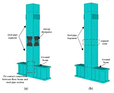
Figure 2. Finite element model, (a) CFST-R, (b) CFST-0.
