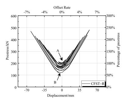
Figure 21. Prestressing—pier top displacement curve.
