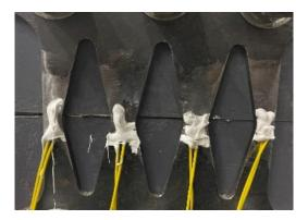
Figure 6. Energy dissipator with strain gauges.
