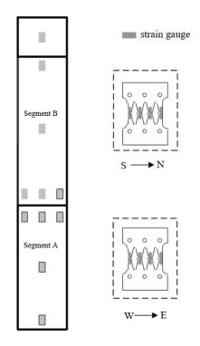
Figure 7. Strain gauge arrangement.
