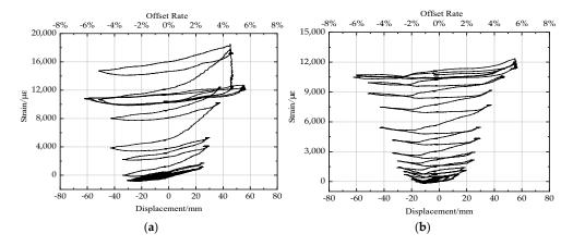
**Figure 20.** CFST-R specimen energy-consuming element strain, (**a**) Strain of East energy-consuming element, (**b**) Strain of West energy dissipation element.
