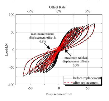
Figure 22. Comparison of hysteresis curves before and after replacement.
