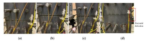
Figure 11. Tension at the joints, (a) Offset rate 2.2%, (b) Offset rate 3.2%, (c) Offset rate 4.2%, (d) Horizontal dislocation at seam.
