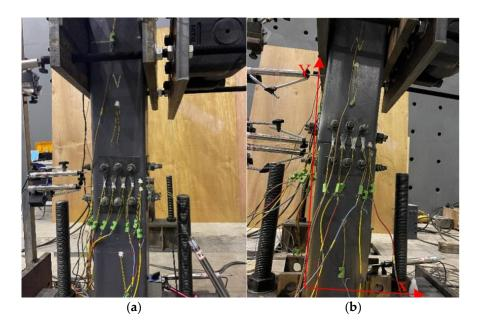
Figure 12. CFST-F loading diagram, (a) Before loading, (b) After loading.
