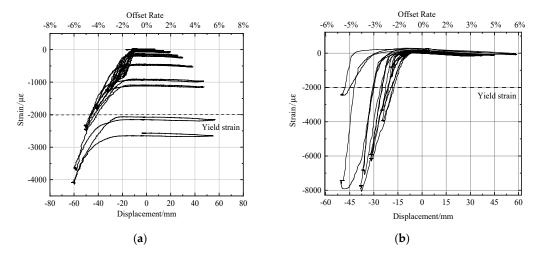
**Figure 19.** Section assembly CFST bridge pier steel pipe part strain, (**a**) CFST-R test specimen, (**b**) CFST-0 test specimen.
