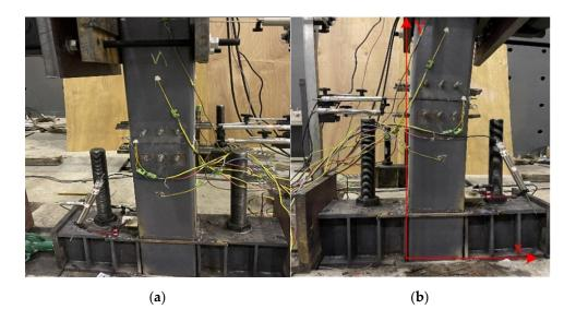
Figure 10. CFST-0 loading diagram, (a) Before loading, (b) After loading.
