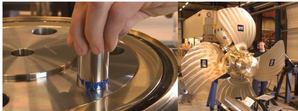
**Figure 1.** Typical application of anaerobic adhesives in propeller blades (securing dowel pins in propeller blades and thread lockers).
