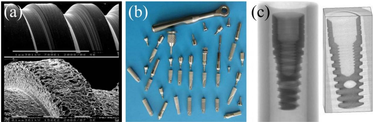
**Figure 23.** SEM images of the NS implant surface after mechanical treatment (a); a set of dental screw intraosseous implants, with instruments and accessories (b); X-ray topographic images of the internal cross-sectional dental implants (c).
