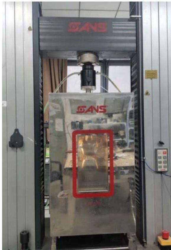
Figure 2. The MTS tensile testing system with a controllable environmental chamber.
