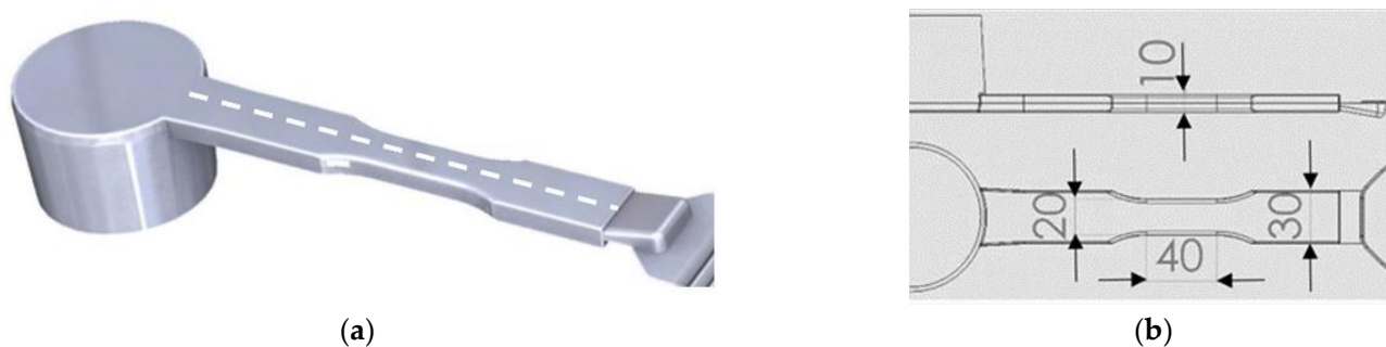
Figure 1. (a) Illustration of the SSM casting and (b) dimensions in mm.
