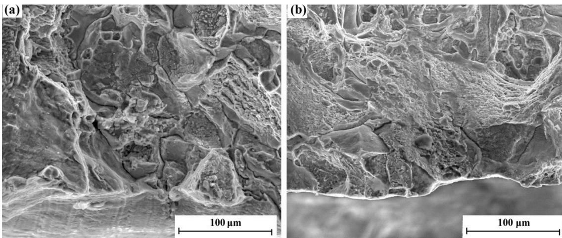
**Figure 2.** The fracture morphology of stress corrosion: (a) 35 °C 3.5 % NaCl solution and (b) 35 °C dry air.
