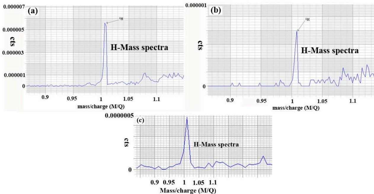
**Figure 6.** The integrated area of H peak: (a) Near the fracture (b) Far from the fracture in simulated working condition, (c) In atmosphere.
