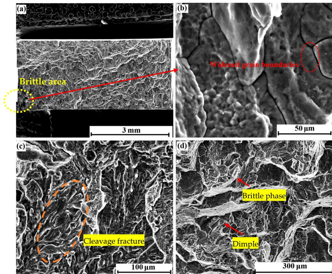
**Figure 4.** Tensile fracture morphology in simulated working condition: (a) The whole morphology, (b) The amplification morphology of the brittle area, (c) The cleavage fracture area (d) The plastic fracture area.
