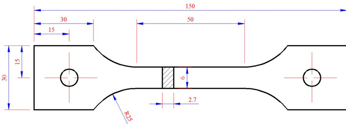
**Figure 1.** Schematic diagram of tensile test specimen (mm).
