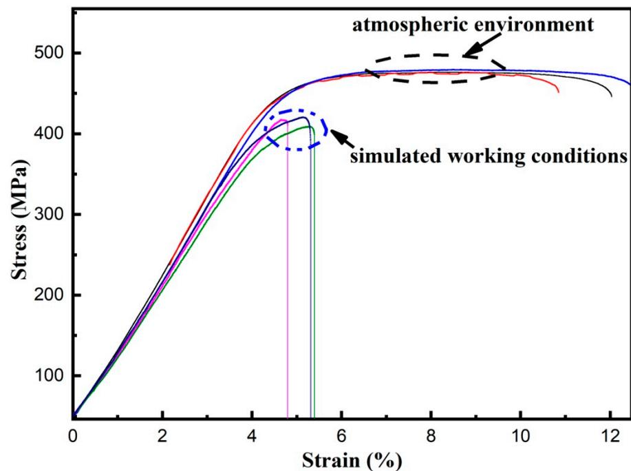
**Figure 3.** The stress-strain curves under different conditions.
