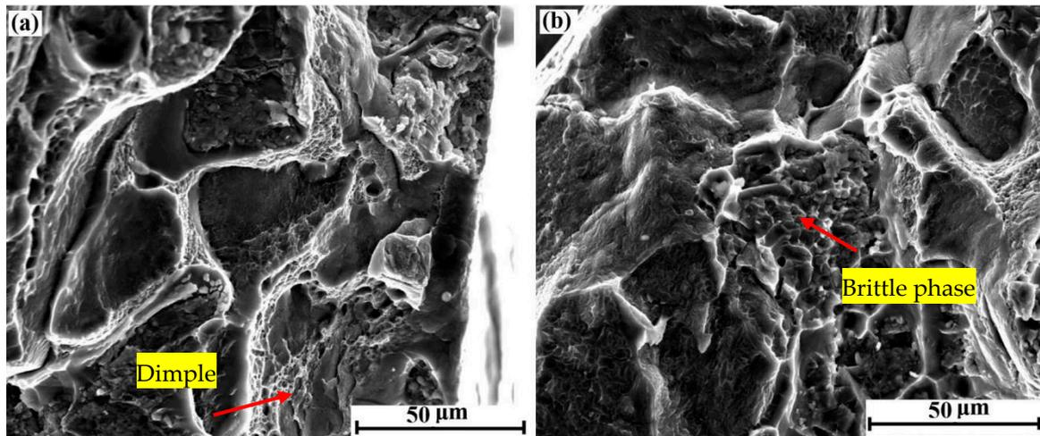
**Figure 5.** Tensile fracture morphology of 7085 specimen in atmosphere: (a) The edge area of fracture and (b) The heart area of fracture.
