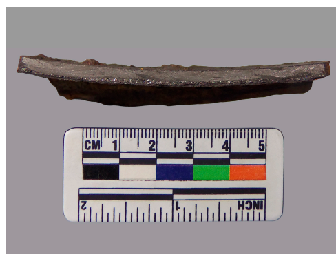
Figure 1. Cross-section appearance of the iron pot sample.
