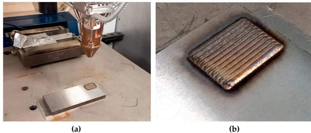
**Figure 1.** (a) Experimental setup for sample manufacturing and (b) the deposited clad for the corrosion analysis.
