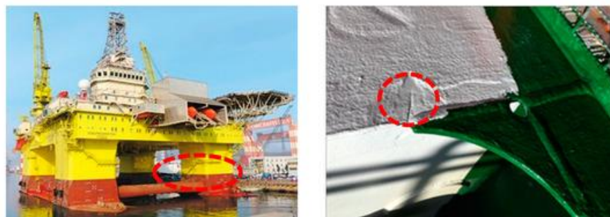
Figure 4. Crack at weld seam of offshore platform [9].
