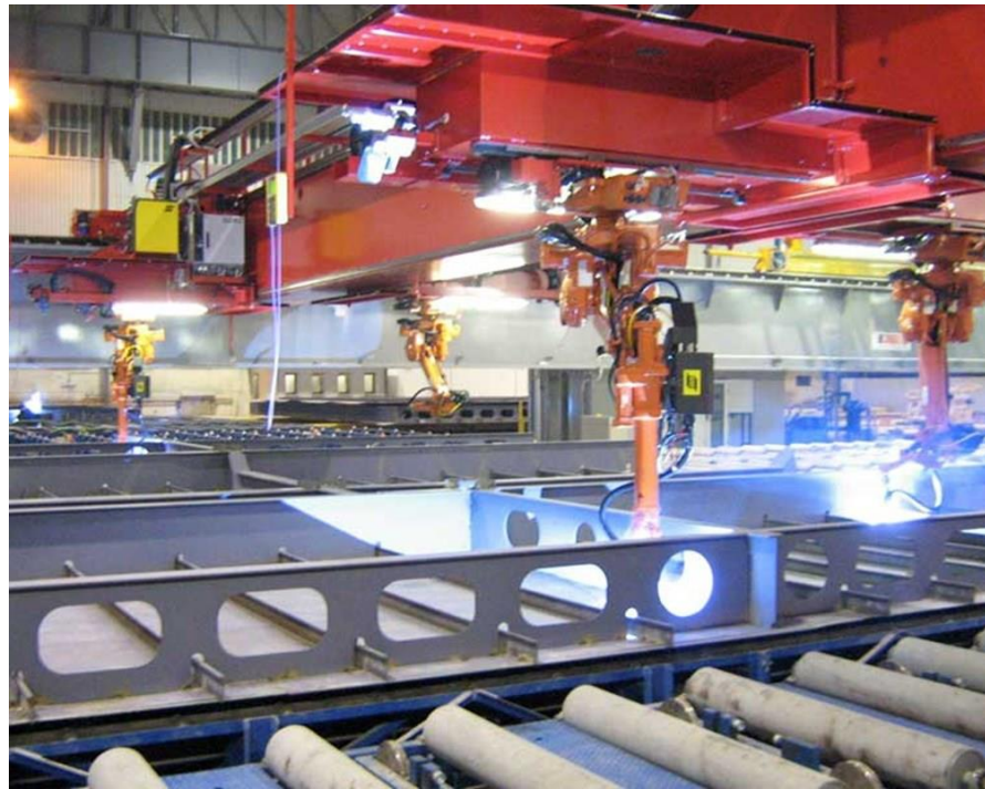
Figure 25. Autonomous welding line robot for shipbuilding ( https://www.kranendonk.com/branches/shipbuilding/ , accessed date 14 May 2022.)
